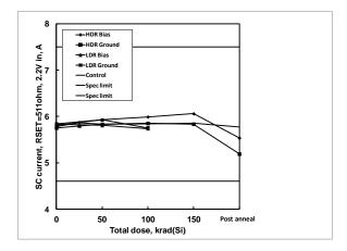
**Figure 54:** ISL75051SEH output short circuit current, RSET=511 $\Omega$ , 2.2V in, as a function of biased and grounded high and low dose rate irradiation and subsequent high temperature accelerated post-high dose rate aging at 100°C. The dose rate was 80 rad(Si)/s. Sample size was 6 for the high dose rate cells and 4 for the low dose rate cells, and three control units were used for the high dose rate test. The specification limits are 4.600A to 7.500A.
