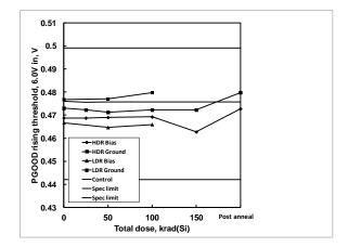
**Figure 43:** ISL75051SEH PGOOD rising threshold, 6.0V in, as a function of biased and grounded high and low dose rate irradiation and subsequent high temperature accelerated post-high dose rate aging at 100°C. The dose rate was 80 rad(Si)/s. Sample size was 6 for the high dose rate cells and 4 for the low dose rate cells, and three control units were used for the high dose rate test. The specification limits are 0.4264V to 0.4836V.
