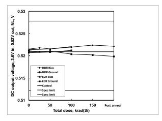
**Figure 14:** ISL75051SEH DC output voltage, 0.52V output, 3.6V input, no load, as a function of biased and grounded high and low dose rate irradiation and subsequent high temperature accelerated post-high dose rate aging at  $100^{\circ}$ C. The dose rate was 80 rad(Si)/s. Sample size was 6 for the high dose rate cells and 4 for the low dose rate cells, and three control units were used for the high dose rate test. The specification limits are 0.5122V – 0.5278V.
