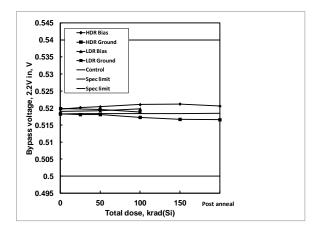
**Figure 34:** ISL75051SEH bypass pin voltage, 2.2V in, as a function of biased and grounded high and low dose rate irradiation and subsequent high temperature accelerated post-high dose rate aging at 100°C. The dose rate was 80 rad(Si)/s. Sample size was 6 for the high dose rate cells and 4 for the low dose rate cells, and three control units were used for the high dose rate test. The specification limits are 0.500V to 0.540V.
