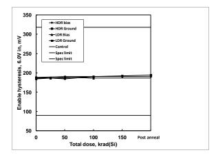
**Figure 10:** ISL75051SEH enable hysteresis, 6.0V input, as a function of biased and grounded high and low dose rate irradiation and subsequent high temperature accelerated post-high dose rate aging at  $100^{\circ}$ C. The dose rate was 80 rad(Si)/s. Sample size was 6 for the high dose rate cells and 4 for the low dose rate cells, and three control units were used for the high dose rate test. The specification limits are 90.0mV – 318.0mV.
