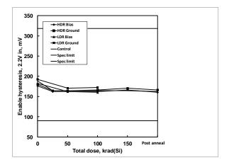
**Figure 7:** ISL75051SEH enable hysteresis, 2.2V input, as a function of biased and grounded high and low dose rate irradiation and subsequent high temperature accelerated post-high dose rate aging at  $100^{\circ}$ C. The dose rate was 80 rad(Si)/s. Sample size was 6 for the high dose rate cells and 4 for the low dose rate cells, and three control units were used for the high dose rate test. The specification limits are 90.0mV – 318.0mV.
