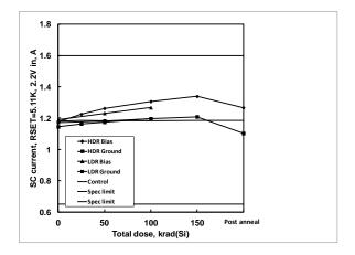
**Figure 53:** ISL75051SEH output short circuit current, 2.2V in, RSET=5.11K, as a function of biased and grounded high and low dose rate irradiation and subsequent high temperature accelerated post-high dose rate aging at 100°C. The dose rate was 80 rad(Si)/s. Sample size was 6 for the high dose rate cells and 4 for the low dose rate cells, and three control units were used for the high dose rate test. The specification limits are 0.650A to 1.600A.
