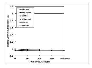
**Figure 2:** ISL75051SEH enable LOW input current as a function of biased and grounded high and low dose rate irradiation and subsequent high temperature accelerated post-high dose rate aging at  $100^{\circ}$ C. The dose rate was 80 rad(Si)/s. Sample size was 6 for the high dose rate cells and 4 for the low dose rate cells, and three control units were used for the high dose rate test. The specification limits are  $-0.100\mu$ A –  $+1.000\mu$ A.
