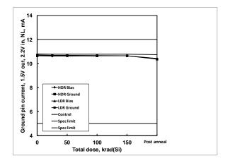
**Figure 35:** ISL75051SEH ground pin current, 1.5V out, 2.2V in, no load, as a function of biased and grounded high and low dose rate irradiation and subsequent high temperature accelerated post-high dose rate aging at 100°C. The dose rate was 80 rad(Si)/s. Sample size was 6 for the high dose rate cells and 4 for the low dose rate cells, and three control units were used for the high dose rate test. The specification limits are 5.000mA to 12.000mA.
