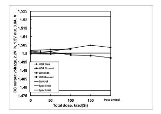
**Figure 17:** ISL75051SEH DC output voltage, 1.5V output, 2.2V input, 3A load, as a function of biased and grounded high and low dose rate irradiation and subsequent high temperature accelerated post-high dose rate aging at  $100^{\circ}$ C. The dose rate was 80 rad(Si)/s. Sample size was 6 for the high dose rate cells and 4 for the low dose rate cells, and three control units were used for the high dose rate test. The specification limits are 1.4780V – 1.5220V.
