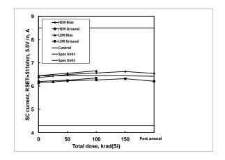
**Figure 56:** ISL75051SEH output short circuit current, RSET=511 $\Omega$ , 6.0V in, as a function of biased and grounded high and low dose rate irradiation and subsequent high temperature accelerated post-high dose rate aging at 100°C. The dose rate was 80 rad(Si)/s. Sample size was 6 for the high dose rate cells and 4 for the low dose rate cells, and three control units were used for the high dose rate test. The specification limits are 4.300A to 8.500A.
