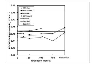
**Figure 47:** ISL75051SEH PGOOD rising threshold, 2.2V in, as a function of biased and grounded high and low dose rate irradiation and subsequent high temperature accelerated post-high dose rate aging at 100°C. The dose rate was 80 rad(Si)/s. Sample size was 6 for the high dose rate cells and 4 for the low dose rate cells, and three control units were used for the high dose rate test. The specification limits are 0.4420V to 0.4992V.
