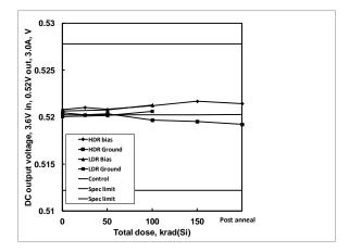
**Figure 15:** ISL75051SEH DC output voltage, 0.52V output, 3.6V input, 3A load, as a function of biased and grounded high and low dose rate irradiation and subsequent high temperature accelerated post-high dose rate aging at  $100^{\circ}$ C. The dose rate was 80 rad(Si)/s. Sample size was 6 for the high dose rate cells and 4 for the low dose rate cells, and three control units were used for the high dose rate test. The specification limits are 0.5122V – 0.5278V.
