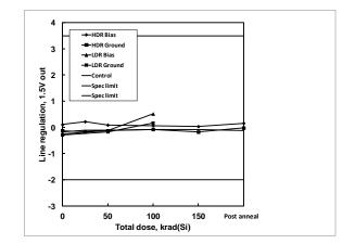
**Figure 28:** ISL75051SEH line regulation, 1.5V out, as a function of biased and grounded high and low dose rate irradiation and subsequent high temperature accelerated post-high dose rate aging at  $100^{\circ}$ C. The dose rate was 80 rad(Si)/s. Sample size was 6 for the high dose rate cells and 4 for the low dose rate cells, and three control units were used for the high dose rate test. The specification limits are -2.000mV – 3.500mV.
