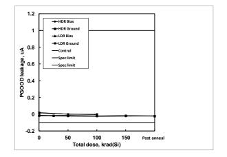
**Figure 40:** ISL75051SEH PGOOD leakage as a function of biased and grounded high and low dose rate irradiation and subsequent high temperature accelerated post-high dose rate aging at  $100^{\circ}$ C. The dose rate was 80 rad(Si)/s. Sample size was 6 for the high dose rate cells and 4 for the low dose rate cells, and three control units were used for the high dose rate test. The specification limits are  $-0.010\mu$ A to  $1.000\mu$ A.
