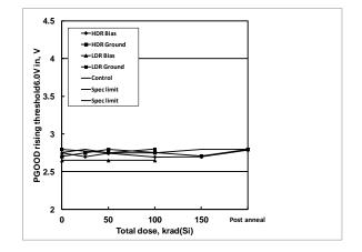
**Figure 48:** ISL75051SEH PGOOD hysteresis, 2.2V in, as a function of biased and grounded high and low dose rate irradiation and subsequent high temperature accelerated post-high dose rate aging at  $100^{\circ}$ C. The dose rate was 80 rad(Si)/s. Sample size was 6 for the high dose rate cells and 4 for the low dose rate cells, and three control units were used for the high dose rate test. The specification limits are 2.500% to 4.000%.
