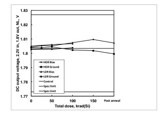
**Figure 20:** ISL75051SEH DC output voltage, 1.8V output, 2.2V input, no load, as a function of biased and grounded high and low dose rate irradiation and subsequent high temperature accelerated post-high dose rate aging at  $100^{\circ}$ C. The dose rate was 80 rad(Si)/s. Sample size was 6 for the high dose rate cells and 4 for the low dose rate cells, and three control units were used for the high dose rate test. The specification limits are 1.7730V – 1.8270V.
