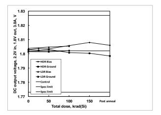
**Figure 21:** ISL75051SEH DC output voltage, 1.8V output, 2.2V input, 3A load, as a function of biased and grounded high and low dose rate irradiation and subsequent high temperature accelerated post-high dose rate aging at  $100^{\circ}$ C. The dose rate was 80 rad(Si)/s. Sample size was 6 for the high dose rate cells and 4 for the low dose rate cells, and three control units were used for the high dose rate test. The specification limits are 1.7730V – 1.8270V.
