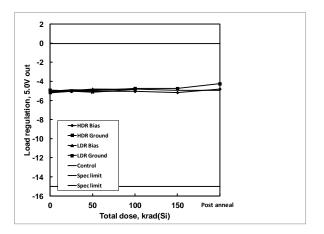
**Figure 33:** ISL75051SEH load regulation, 5.0V out, as a function of biased and grounded high and low dose rate irradiation and subsequent high temperature accelerated post-high dose rate aging at  $100^{\circ}$ C. The dose rate was 80 rad(Si)/s. Sample size was 6 for the high dose rate cells and 4 for the low dose rate cells, and three control units were used for the high dose rate test. The specification limits are -15.000mV to -0.050mV.
