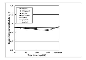
**Figure 8:** ISL75051SEH enable rising threshold, 6.0V input, as a function of biased and grounded high and low dose rate irradiation and subsequent high temperature accelerated post-high dose rate aging at  $100^{\circ}$ C. The dose rate was 80 rad(Si)/s. Sample size was 6 for the high dose rate cells and 4 for the low dose rate cells, and three control units were used for the high dose rate test. The specification limits are 0.600V – 1.200V.
