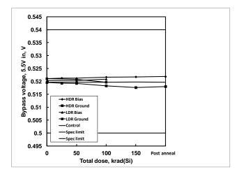
**Figure 37:** ISL75051SEH bypass pin voltage, 6.0V in, as a function of biased and grounded high and low dose rate irradiation and subsequent high temperature accelerated post-high dose rate aging at 100°C. The dose rate was 80 rad(Si)/s. Sample size was 6 for the high dose rate cells and 4 for the low dose rate cells, and three control units were used for the high dose rate test. The specification limits are 0.500V to 0.540V.
