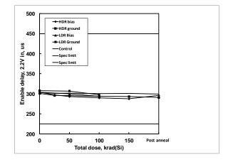
**Figure 11:** ISL75051SEH enable propagation delay, 2.2V input, as a function of biased and grounded high and low dose rate irradiation and subsequent high temperature accelerated post-high dose rate aging at  $100^{\circ}$ C. The dose rate was 80 rad(Si)/s. Sample size was 6 for the high dose rate cells and 4 for the low dose rate cells, and three control units were used for the high dose rate test. The specification limits are  $225\mu s - 450\mu s$ .
