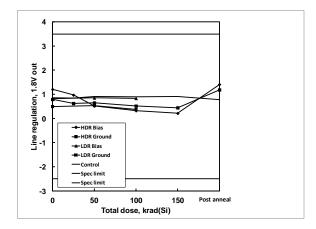
**Figure 30:** ISL75051SEH line regulation, 1.8V out, as a function of biased and grounded high and low dose rate irradiation and subsequent high temperature accelerated post-high dose rate aging at  $100^{\circ}$ C. The dose rate was 80 rad(Si)/s. Sample size was 6 for the high dose rate cells and 4 for the low dose rate cells, and three control units were used for the high dose rate test. The specification limits are -2.500mV to +3.500mV.
