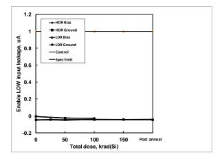
**Figure 3:** ISL75051SEH enable HIGH input current as a function of biased and grounded high and low dose rate irradiation and subsequent high temperature accelerated post-high dose rate aging at  $100^{\circ}$ C. The dose rate was 80 rad(Si)/s. Sample size was 6 for the high dose rate cells and 4 for the low dose rate cells, and three control units were used for the high dose rate test. The specification limits are  $-0.100\mu$ A –  $+1.000\mu$ A.
