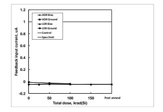
**Figure 4:** ISL75051SEH feedback pin input current as a function of biased and grounded high and low dose rate irradiation and subsequent high temperature accelerated post-high dose rate aging at  $100^{\circ}$ C. The dose rate was 80 rad(Si)/s. Sample size was 6 for the high dose rate cells and 4 for the low dose rate cells, and three control units were used for the high dose rate test. The specification limits are -1.00µA – +1.00µA.
