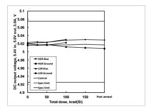
**Figure 25:** ISL75051SEH DC output voltage, 5.0V output, 5.4V input, 3A load, as a function of biased and grounded high and low dose rate irradiation and subsequent high temperature accelerated post-high dose rate aging at  $100^{\circ}$ C. The dose rate was 80 rad(Si)/s. Sample size was 6 for the high dose rate cells and 4 for the low dose rate cells, and three control units were used for the high dose rate test. The specification limits are 4.9250V - 5.0750V.
