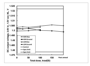
**Figure 18:** ISL75051SEH DC output voltage, 1.5V output, 3.6V input, no load, as a function of biased and grounded high and low dose rate irradiation and subsequent high temperature accelerated post-high dose rate aging at  $100^{\circ}$ C. The dose rate was 80 rad(Si)/s. Sample size was 6 for the high dose rate cells and 4 for the low dose rate cells, and three control units were used for the high dose rate test. The specification limits are 1.4780V – 1.5220V.
