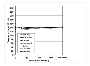
**Figure 50:** ISL75051SEH dropout voltage, 2.5V out, 2A load current, as a function of biased and grounded high and low dose rate irradiation and subsequent high temperature accelerated post-high dose rate aging at 100°C. The dose rate was 80 rad(Si)/s. Sample size was 6 for the high dose rate cells and 4 for the low dose rate cells, and three control units were used for the high dose rate test. The specification limits are 70.000mV to 200.000mV.
