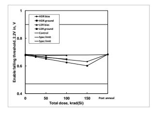
**Figure 6:** ISL75051SEH enable falling threshold, 2.2V input, as a function of biased and grounded high and low dose rate irradiation and subsequent high temperature accelerated post-high dose rate aging at  $100^{\circ}$ C. The dose rate was 80 rad(Si)/s. Sample size was 6 for the high dose rate cells and 4 for the low dose rate cells, and three control units were used for the high dose rate test. The specification limits are 0.470V - 0.900V.
