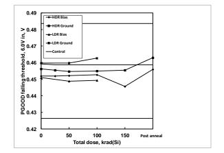
**Figure 44:** ISL75051SEH PGOOD falling threshold, 6.0V in, as a function of biased and grounded high and low dose rate irradiation and subsequent high temperature accelerated post-high dose rate aging at 100°C. The dose rate was 80 rad(Si)/s. Sample size was 6 for the high dose rate cells and 4 for the low dose rate cells, and three control units were used for the high dose rate test. The specification limits are 0.4420V to 0.4992V.
