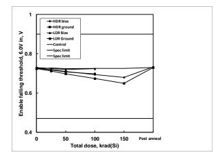
**Figure 9:** ISL75051SEH enable falling threshold, 6.0V input, as a function of biased and grounded high and low dose rate irradiation and subsequent high temperature accelerated post-high dose rate aging at  $100^{\circ}$ C. The dose rate was 80 rad(Si)/s. Sample size was 6 for the high dose rate cells and 4 for the low dose rate cells, and three control units were used for the high dose rate test. The specification limits are 0.470V – 0.900V.
