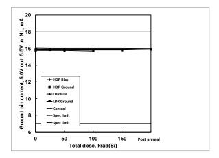
**Figure 38:** ISL75051SEH ground pin current, 1.5V out, 6.0V in, no load, as a function of biased and grounded high and low dose rate irradiation and subsequent high temperature accelerated post-high dose rate aging at 100°C. The dose rate was 80 rad(Si)/s. Sample size was 6 for the high dose rate cells and 4 for the low dose rate cells, and three control units were used for the high dose rate test. The specification limits are 7.000mA to 18.000mA.
