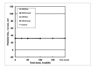
**Figure 41:** ISL75051SEH PGOOD output LOW voltage, 1mA, as a function of biased and grounded high and low dose rate irradiation and subsequent high temperature accelerated post-high dose rate aging at 100°C. The dose rate was 80 rad(Si)/s. Sample size was 6 for the high dose rate cells and 4 for the low dose rate cells, and three control units were used for the high dose rate test. The specification limits are 0mV to 100.0mV.
