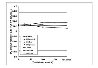
**Figure 24:** ISL75051SEH DC output voltage, 5.0V output, 5.4V input, 3A load, as a function of biased and grounded high and low dose rate irradiation and subsequent high temperature accelerated post-high dose rate aging at  $100^{\circ}$ C. The dose rate was 80 rad(Si)/s. Sample size was 6 for the high dose rate cells and 4 for the low dose rate cells, and three control units were used for the high dose rate test. The specification limits are 4.9250V - 5.0750V.
