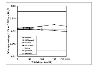
**Figure 12:** ISL75051SEH DC output voltage, 0.52V output, 2.2V input, no load, as a function of biased and grounded high and low dose rate irradiation and subsequent high temperature accelerated post-high dose rate aging at  $100^{\circ}$ C. The dose rate was 80 rad(Si)/s. Sample size was 6 for the high dose rate cells and 4 for the low dose rate cells, and three control units were used for the high dose rate test. The specification limits are 0.5122V – 0.5278V.
