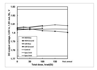
**Figure 22:** ISL75051SEH DC output voltage, 1.8V output, 3.6V input, no load, as a function of biased and grounded high and low dose rate irradiation and subsequent high temperature accelerated post-high dose rate aging at  $100^{\circ}$ C. The dose rate was 80 rad(Si)/s. Sample size was 6 for the high dose rate cells and 4 for the low dose rate cells, and three control units were used for the high dose rate test. The specification limits are 1.7730V – 1.8270V.
