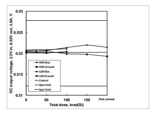
**Figure 13:** ISL75051SEH DC output voltage, 0.52V output, 2.2V input, 3A load, as a function of biased and grounded high and low dose rate irradiation and subsequent high temperature accelerated post-high dose rate aging at  $100^{\circ}$ C. The dose rate was 80 rad(Si)/s. Sample size was 6 for the high dose rate cells and 4 for the low dose rate cells, and three control units were used for the high dose rate test. The specification limits are 0.5122V – 0.5278V.
