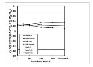
**Figure 27:** ISL75051SEH DC output voltage, 5.0V output, 6.0V input, 3A load, as a function of biased and grounded high and low dose rate irradiation and subsequent high temperature accelerated post-high dose rate aging at 100°C. The dose rate was 80 rad(Si)/s. Sample size was 6 for the high dose rate cells and 4 for the low dose rate cells, and three control units were used for the high dose rate test. The specification limits are 4.9250V – 5.0750V.
