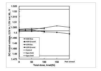
**Figure 16:** ISL75051SEH DC output voltage, 1.5V output, 2.2V input, no load, as a function of biased and grounded high and low dose rate irradiation and subsequent high temperature accelerated post-high dose rate aging at  $100^{\circ}$ C. The dose rate was 80 rad(Si)/s. Sample size was 6 for the high dose rate cells and 4 for the low dose rate cells, and three control units were used for the high dose rate test. The specification limits are 1.4780V – 1.5220V.
