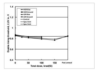
**Figure 5:** ISL75051SEH enable rising threshold, 2.2V input, as a function of biased and grounded high and low dose rate irradiation and subsequent high temperature accelerated post-high dose rate aging at  $100^{\circ}$ C. The dose rate was 80 rad(Si)/s. Sample size was 6 for the high dose rate cells and 4 for the low dose rate cells, and three control units were used for the high dose rate test. The specification limits are 0.600V - 1.200V.
