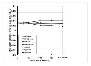
**Figure 26:** ISL75051SEH DC output voltage, 5.0V output, 6.0V input, no load, as a function of biased and grounded high and low dose rate irradiation and subsequent high temperature accelerated post-high dose rate aging at  $100^{\circ}$ C. The dose rate was 80 rad(Si)/s. Sample size was 6 for the high dose rate cells and 4 for the low dose rate cells, and three control units were used for the high dose rate test. The specification limits are 4.9250V - 5.0750V.
