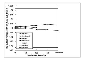
**Figure 19:** ISL75051SEH DC output voltage, 1.5V output, 3.6V input, 3A load, as a function of biased and grounded high and low dose rate irradiation and subsequent high temperature accelerated post-high dose rate aging at  $100^{\circ}$ C. The dose rate was 80 rad(Si)/s. Sample size was 6 for the high dose rate cells and 4 for the low dose rate cells, and three control units were used for the high dose rate test. The specification limits are 1.4780V – 1.5220V.
