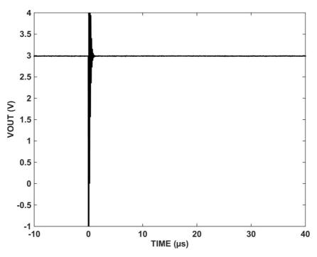
Figure 2. Example of a Spike SET for ISL71610SLHM with 0mA Input and 3V Supply
