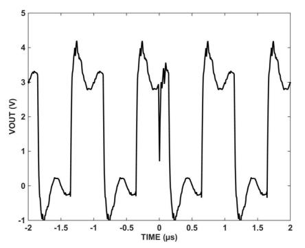
Figure 7. Example of a dynamic SET capture for the ISL71710SLHM operating at 1MHz at 3V and irradiated with praseodymium (60MeV·cm2/mg).
