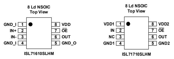
Figure 1. ISL71610SLHM and ISL71710SLHM Pin Assignments
