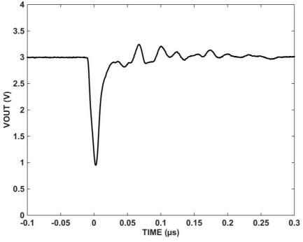
Figure 6. Expanded SET for ISL71710SLHM with IN = 2.4V and VDD1 = VDD2 = 3V with normal incidence praseodymium for 60MeV·cm2/mg.
