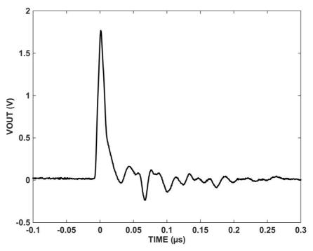
Figure 5. Expanded SET for ISL71710SLHM with IN = 0.8V and VDD1 = VDD2 = 3V with normal incidence praseodymium for 60MeV·cm<sup>2</sup>/mg
