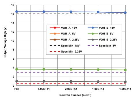
Figure 2. ISL70219ASEH Output Voltage High ( $V_{OH}$ ), Channels A and B, with  $V_S$  = ±18V, ±5V, and ±2.25V,  $R_L$  = 2k $\Omega$ , following irradiation to each level. The error bars (if visible) represent the minimum and maximum measured values. The SMD limits are 16V minimum for  $V_S$  = ±18V, 3V minimum for  $V_S$  = ±5V, and 0.45V minimum for  $V_S$  = ±2.25V.
