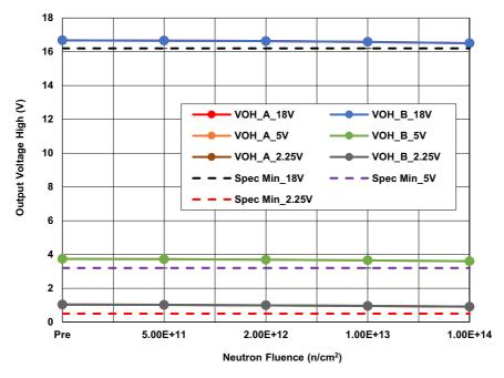
Figure 1. ISL70219ASEH Output Voltage High ( $V_{OH}$ ), Channels A and B, with  $V_S = \pm 18V, \pm 5V$ , and  $\pm 2.25V$ ,  $R_L = 10k\Omega$ , following irradiation to each level. The error bars (if visible) represent the minimum and maximum measured values. The SMD limits are 16.2V minimum for  $V_S = \pm 18V$ , 3.2V minimum for  $V_S = \pm 5V$ , and 0.5V minimum for  $V_S = \pm 2.25V$ .
