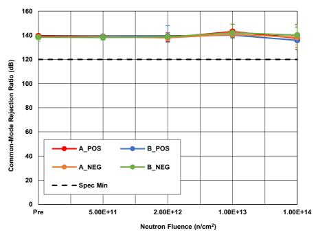
Figure 15. ISL70219ASEH Common-Mode Rejection Ratio (CMRR), Channels A and B, with  $V_S$  = ±18V, following irradiation to each level. The error bars (if visible) represent the minimum and maximum measured values. The SMD limit is 120dB minimum.
