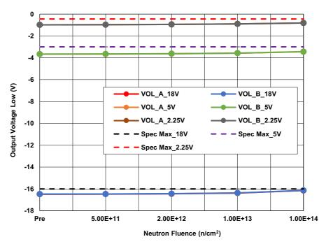
Figure 4. ISL70219ASEH Output Voltage Low ( $V_{OL}$ ), Channels A and B, with  $V_S$  = ±18V, ±5V, and ±2.25V,  $R_L$  = 2k $\Omega$ , following irradiation to each level. The error bars (if visible) represent the minimum and maximum measured values. The SMD limits are -16V maximum for  $V_S$  = ±18V, -3V maximum for  $V_S$  = ±5V, and -0.45V maximum for  $V_S$  = ±2.25V.
