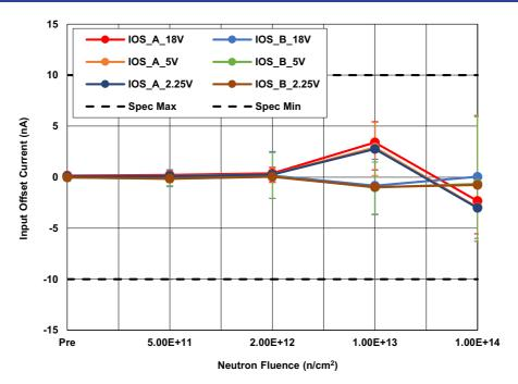
Figure 10. ISL70219ASEH Input Offset Current ( $I_{OS}$ ), Channels A and B, with  $V_S$  = ±18V, ±5V, and ±2.25V, following irradiation to each level. The error bars (if visible) represent the minimum and maximum measured values. The SMD limits are -10nA minimum and 10nA maximum.
