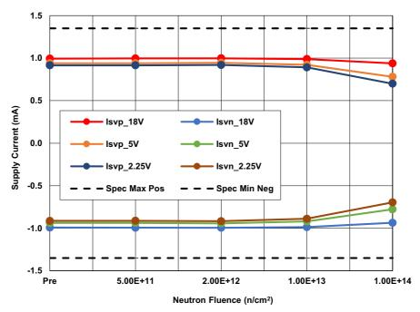
Figure 5. ISL70219ASEH Positive and Negative Supply Current ( $I_{SVP}$  and  $I_{SVN}$ ), for Channels A + B, with  $V_S$  = ±18V, ±5V, and ±2.25V, following irradiation to each level. The error bars (if visible) represent the minimum and maximum measured values. The SMD limits are -1.35mA minimum and 1.35mA maximum.
