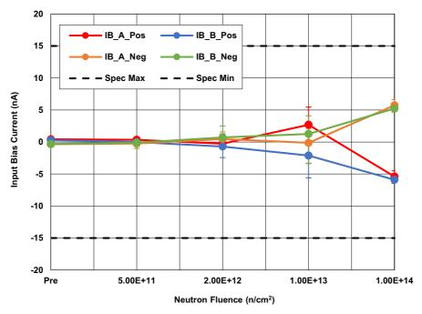
Figure 9. ISL70219ASEH Input Bias Current ( $I_B$ ), Channels A and B, with  $V_S$  = ±2.25V, following irradiation to each level. The error bars (if visible) represent the minimum and maximum measured values. The SMD limits are -15nA minimum and 15nA maximum.
