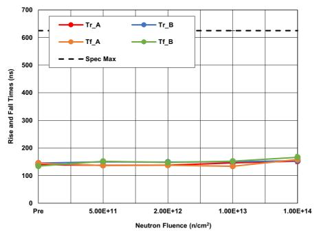
Figure 19. ISL70219ASEH Rise Time  $(t_r)$  and Fall Time  $(t_f)$ , Channels A and B, with  $V_S = \pm 18V$ , following irradiation to each level. The error bars (if visible) represent the minimum and maximum measured values. The SMD limit is 625ns maximum.
