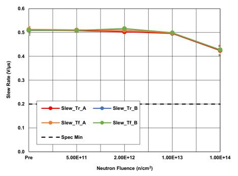
Figure 18. ISL70219ASEH Slew Rate (SR), Channels A and B, with  $V_S = \pm 18V$ ,  $A_V = 1$ ,  $R_L = 2k\Omega$ , following irradiation to each level. The error bars (if visible) represent the minimum and maximum measured values. The SMD limit is  $0.2V/\mu s$  minimum.
