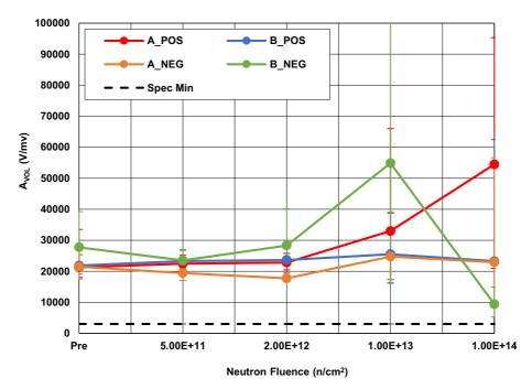
Figure 11. ISL70219ASEH Open-Loop Gain ( $A_{VOL}$ ), Channels A and B, with  $V_S$  = ±18V, following irradiation to each level. The error bars (if visible) represent the minimum and maximum measured values. The SMD limit is 3000V/mV minimum.
