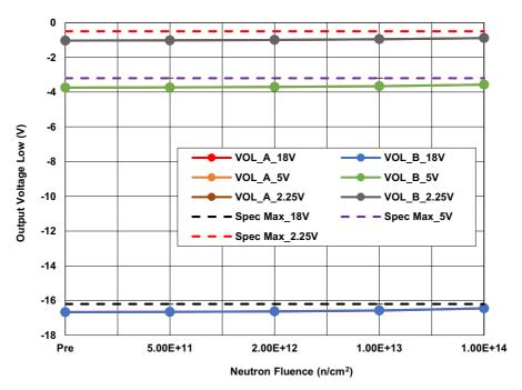
Figure 3. ISL70219ASEH Output Voltage Low ( $V_{OL}$ ), Channels A and B, with  $V_S$  = ±18V, ±5V, and ±2.25V,  $R_L$  = 10k $\Omega$ , following irradiation to each level. The error bars (if visible) represent the minimum and maximum measured values. The SMD limits are -16.2V maximum for  $V_S$  = ±18V, -3.2V maximum for  $V_S$  = ±5V, and -0.5V maximum for  $V_S$  = ±2.25V.
