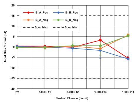
Figure 8. ISL70219ASEH Input Bias Current ( $I_B$ ), Channels A and B, with  $V_S = \pm 5V$ , following irradiation to each level. The error bars (if visible) represent the minimum and maximum measured values. The SMD limits are -15nA minimum and 15nA maximum.
