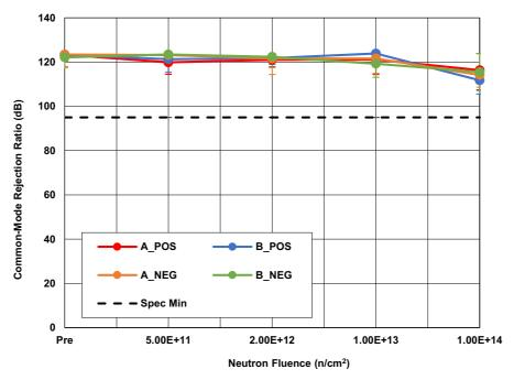
Figure 17. ISL70219ASEH Common-Mode Rejection Ratio (CMRR), Channels A and B, with  $V_S$  =  $\pm 2.25V$ , following irradiation to each level. The error bars (if visible) represent the minimum and maximum measured values. The SMD limit is 95dB minimum.
