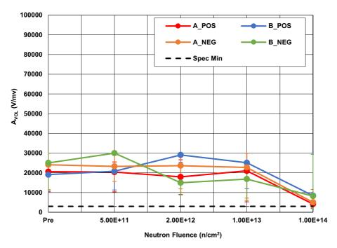
Figure 12. ISL70219ASEH Open-Loop Gain ( $A_{VOL}$ ), Channels A and B, with  $V_S$  = ±5V, following irradiation to each level. The error bars (if visible) represent the minimum and maximum measured values. The SMD limit is 3000V/mV minimum.
