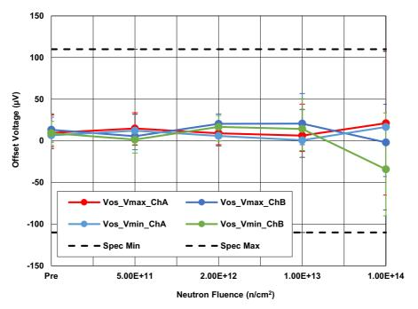
Figure 6. ISL70219ASEH Input Offset Voltage ( $V_{OS}$ ), Channels A and B, with  $V_S$  = ±18V and ±2.25V, following irradiation to each level. The error bars (if visible) represent the minimum and maximum measured values. The SMD limits -110 $\mu$ V minimum and 110 $\mu$ V maximum.
