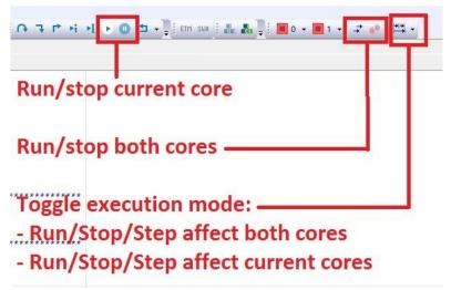
Figure 2-6: Multicore Debug Interface
