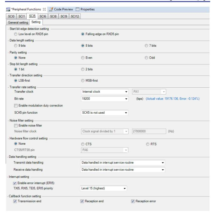
Figure 4-13 SCI5 Asynchronous Setting
