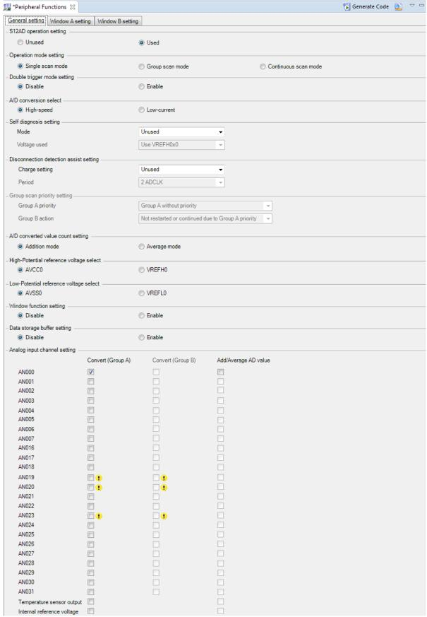
Figure 4-8 A/D Converter tab-1
