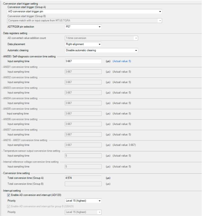
Figure 4-9 A/D Converter tab-2
