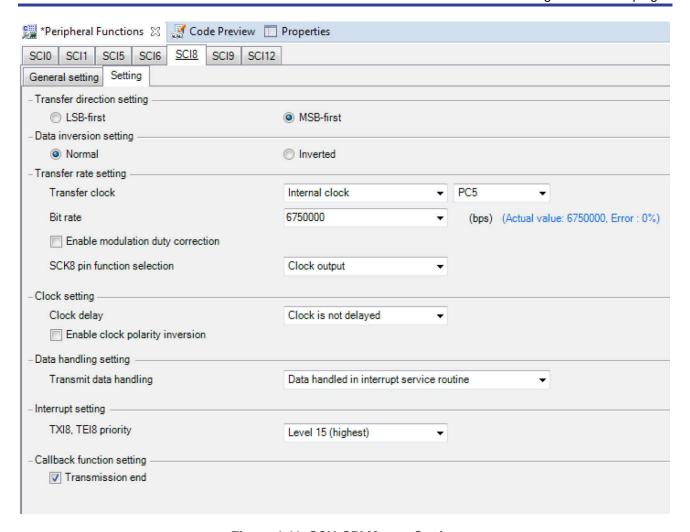
Figure 4-11 SCI8 SPI Master Setting
