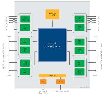
Embedded applications further benefit from the ability of the Tsi576 to route packets to multiple endpoints through hierarchical lookup tables, independent unicast and multicast routing mechanisms, and error management extensions that provide proactive issue notification to the fabric controller. In addition, the Tsi576 supports both in-band serial RapidIO access and out-of-band access to the full fabric register set through the I<sup>2</sup>C interface.
