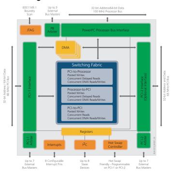
The high level of performance and flexibility of the PowerSpan II is made possible through Switched PCI - unique to PowerSpan II. Switched PCI uses a switching fabric to enable data streams to pass from port-to-port across the multi-ported PowerSpan II without collision. This improves the burst performance and decreases latency on the PCI and processor buses — a key element in enabling increased I/O performance.
