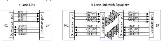
A group of Transmitters and Receivers located on the same component that operate together. Two ports form the ends of a serial communications link. A four-port Retimer that supports two independent links, each with 4 lanes, is
