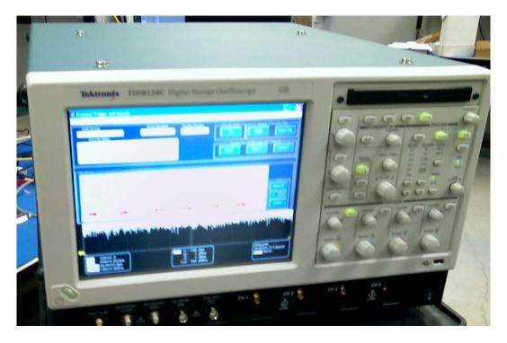
The latency measurements were made using a Tektronix TDS6124C oscilloscope. This scope has a 12-GHz bandwidth, 20-GSps sample rate, and 32 MB of storage on each of its four channels. It also has the Protocol Triggering and Decoding Software, which can easily decode the 8b/10b serial data streams, and set serial pattern markers after capture.
