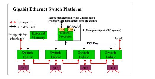
Figure 3: Gigabit Ethernet Application Example
