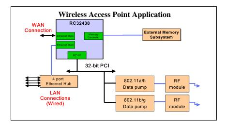
Figure 5: Wireless Access Point Application Example
