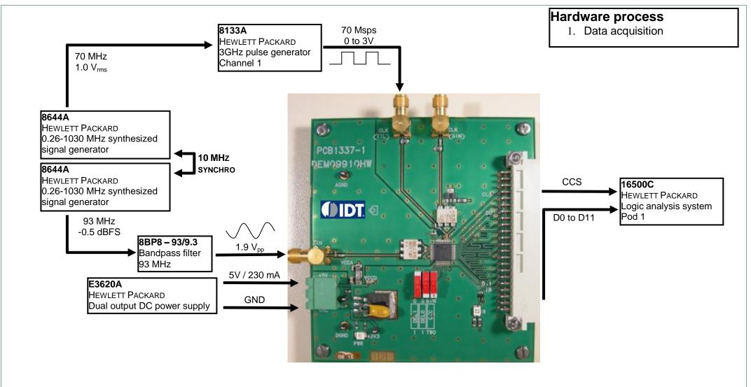
Fig 2. ADC1207S080 hardware setup
