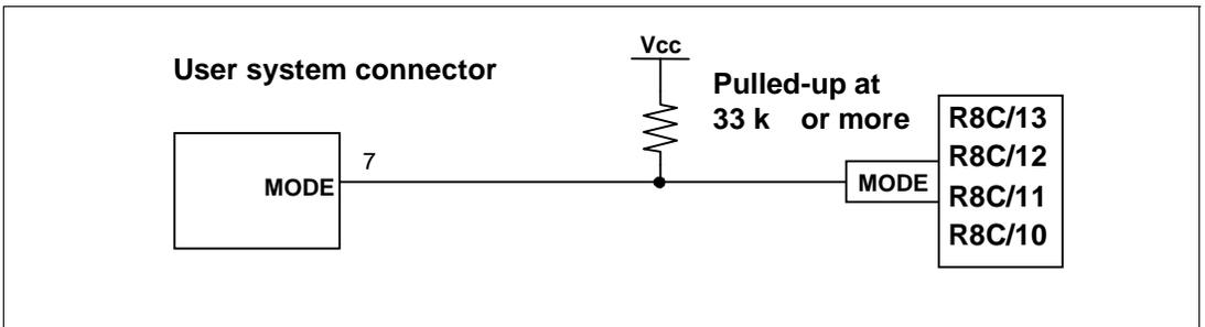
**Figure 3.3 Connection of E7 Emulator and MODE Pin**
