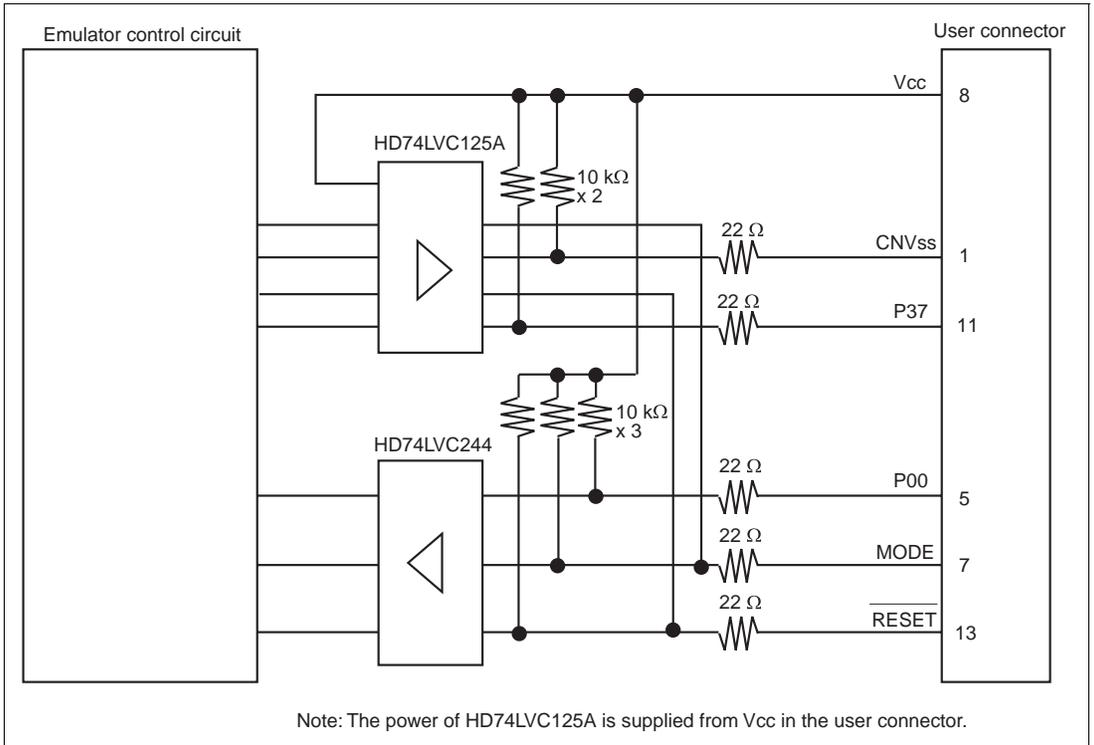
**Figure 3.6 Interface Circuit in the Emulator (Reference)**
