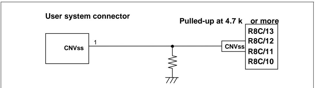
**Figure 3.4 Connection of E7 Emulator and CNVss Pin**
