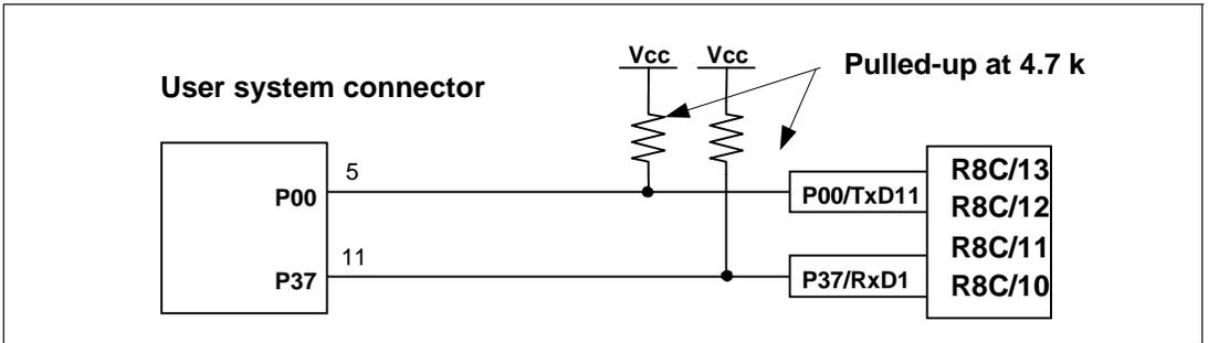
**Figure 3.2 Connection of E7 Emulator and MCU**
