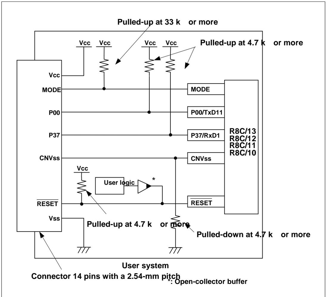
**Figure 3.1 Example of E7 Connection**
