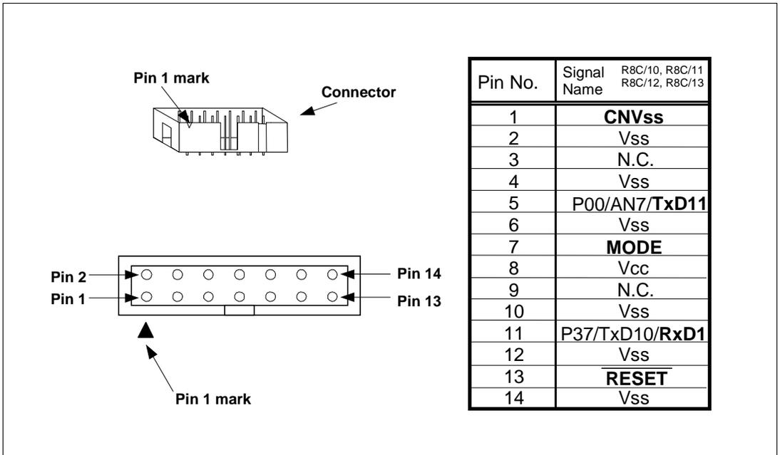
Figure 2.1 Pin Assignments of the E7 Connector
