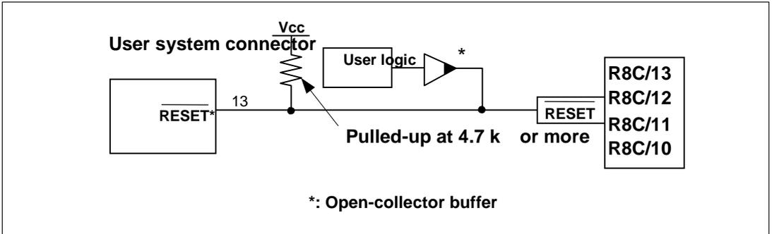
**Figure 3.5 Example of a Reset Circuit**
