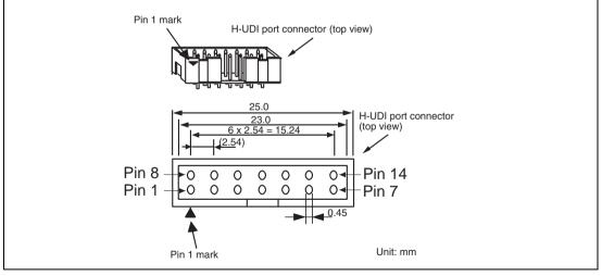
Figure 1.1 Pin Assignments of the H-UDI Port Connector (14 Pins)
