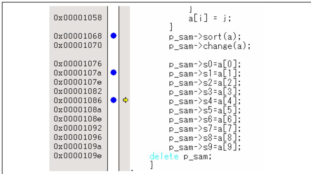
**Figure 2.1 [Source] Window at Execution Halted (Sequential Break)**
