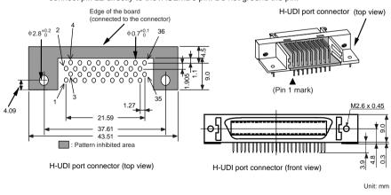
Figure 1.1 Pin Assignments of the H-UDI Port Connector (36 Pins)
