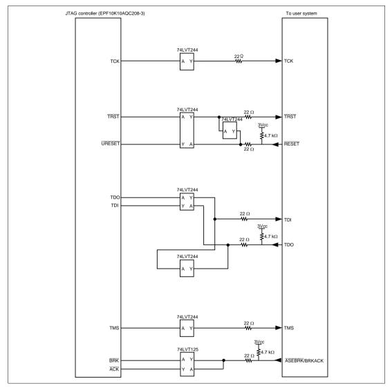
Figure 6.8 User System Interface Circuit of the Hitachi-UDI Pin (HS7760KCI02H) (Model Name: HS0005KCI04H)
