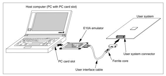
Figure 6.1 Connecting Ferrite Core
