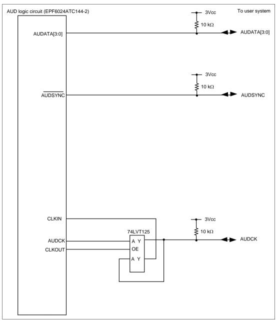
Figure 6.6 User System Interface Circuit of the AUD Pin (HS7760KCM02H) (Model Name: HS0005KCM04H)
