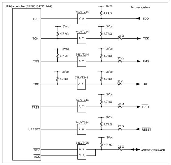
Figure 6.4 User System Interface Circuit (HS7760KCM01H) (Model Name: HS0005KCM03H)
