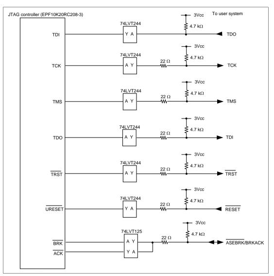
Figure 6.7 shows the user system interface circuit of the emulator (HS7760KCI01H).
