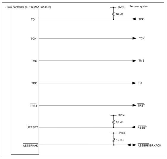
Figure 6.5 User System Interface Circuit of the Hitachi-UDI Pin (HS7760KCM02H) (Model Name: HS0005KCM04H)
