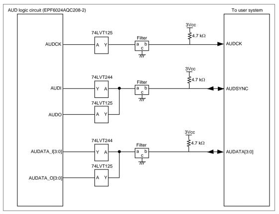
Figure 6.9 User System Interface Circuit of the AUD Pin (HS7760KCI02H) (Model Name: HS0005KCI04H)
