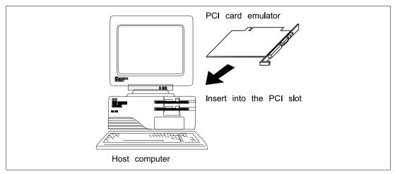
Figure 2.3 Inserting the PCI Card Emulator in the Host Computer's Slot
