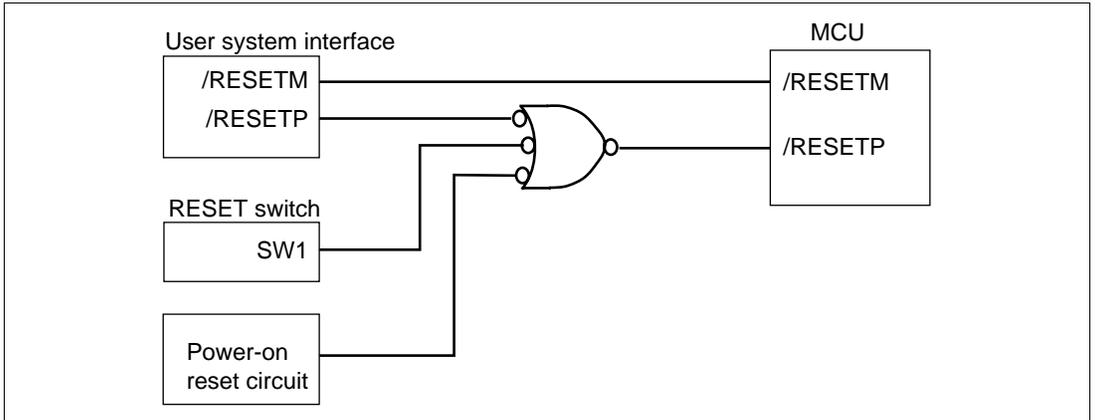
**Figure 4.3 Reset Circuit Logic Diagram**
