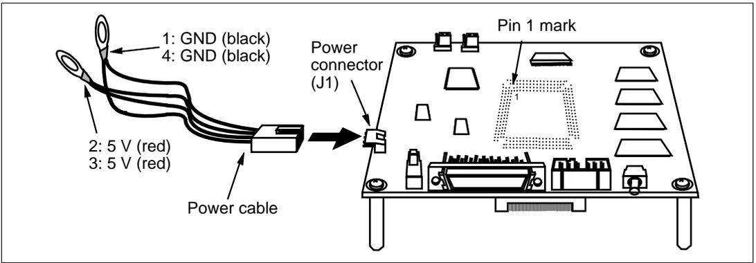
**Figure 5.4 Connecting Power Cables to Power Connector**
