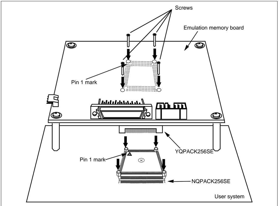
**Figure 5.2 Connecting Emulation Memory Board to User System**
