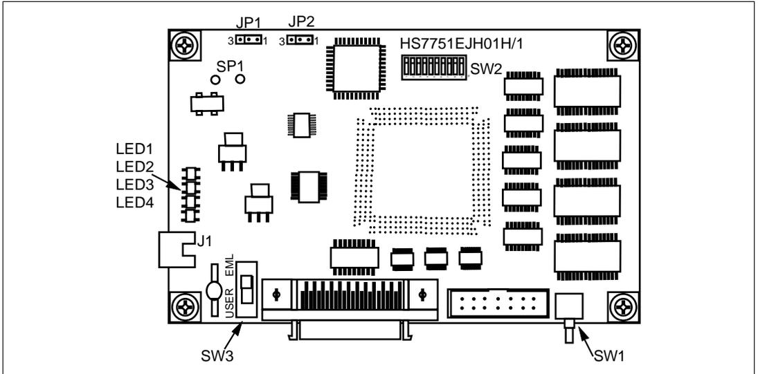
**Figure 4.1** Switches, Socket, and LEDs
