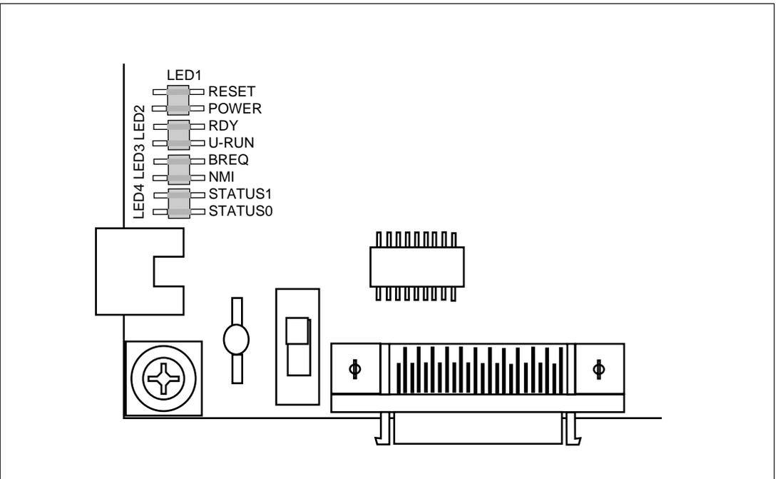
**Figure 4.4 LED Location and Indication on the Board**
