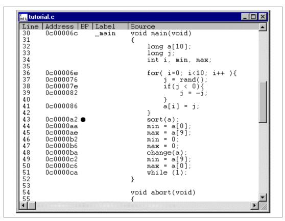
Figure 3.10 [Source] Window (Setting a Software Breakpoint)
