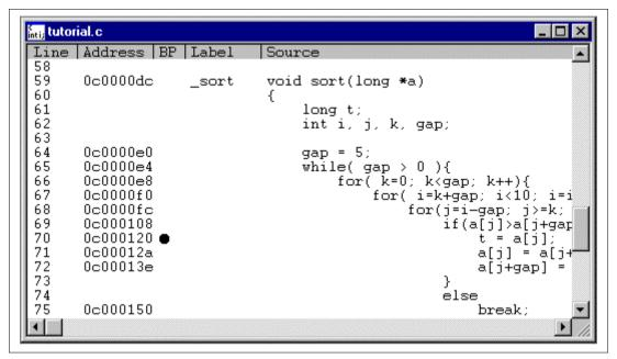
Figure 3.59 [Source] Window (Software Breakpoint Setting)
