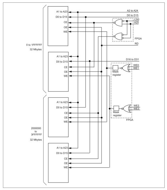
Figure 6.10 Flash Memory Wiring
