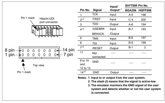
Figure 6.1 Pin Arrangement of the Hitachi-UDI Port Connector (14 Pins)
