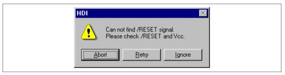
Figure 2.12 [Can not find /RESET signal] Dialog Box
