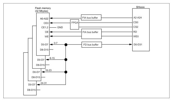
Figure 3.69 Flash Memory Wiring
