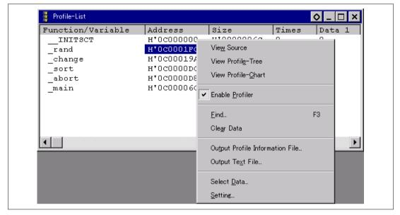
Figure 3.62 Selection of [Enable Profiler]
