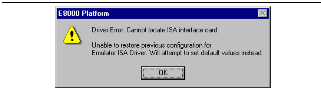
Figure 3.27 Error Message on PC Interface Board Connection Failure
