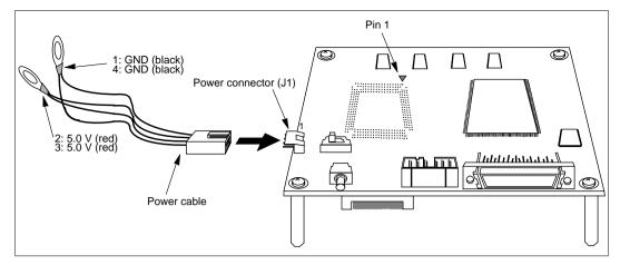
Figure 5.4 Connecting Power Cables to Power Connector
