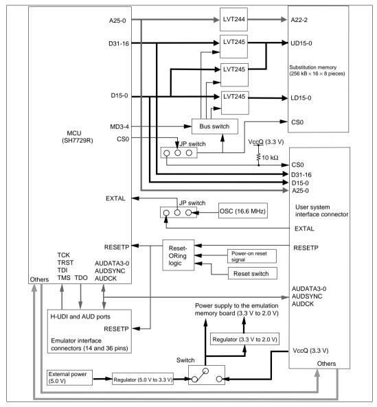
Figure 8.1 Emulation Memory Board Block Diagram
