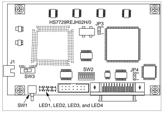
Figure 4.1 Switches and LEDs
