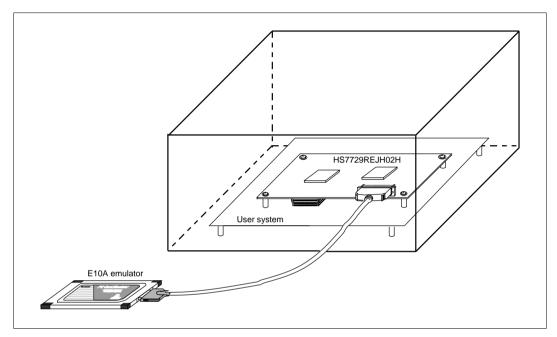
Figure 9.1 Configuration for Countermeasure against EMI Noise
