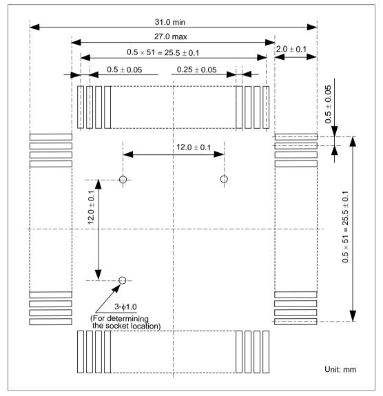
Figure 5.7 Recommended Dimensions for Mount Pad
