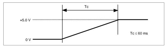
Figure 5.5 Characteristics of DC Rising Timing
