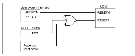
Figure 4.3 Reset Circuit Logic Diagram
