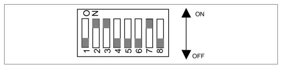
Figure 4.2 DIP Switch (SW2) Appearance and Settings at Shipment
