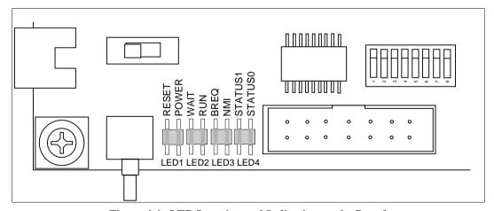
Figure 4.4 LED Location and Indication on the Board
