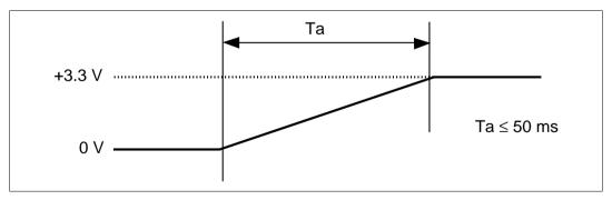
Figure 5.3 Characteristics of DC Rising Timing
