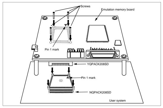
Figure 5.2 Connecting Emulation Memory Board to User System
