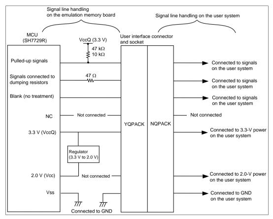
Figure 7.1 Signal Line Handling on the Emulation Memory Board and User System
