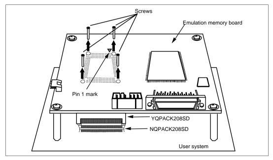
Figure 5.6 Disconnecting Emulation Memory Board
