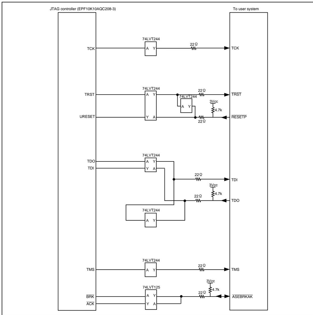
**Figure 6.8 User System Interface Circuit of the Hitachi-UDI Pin (HS7727KCI02H)
