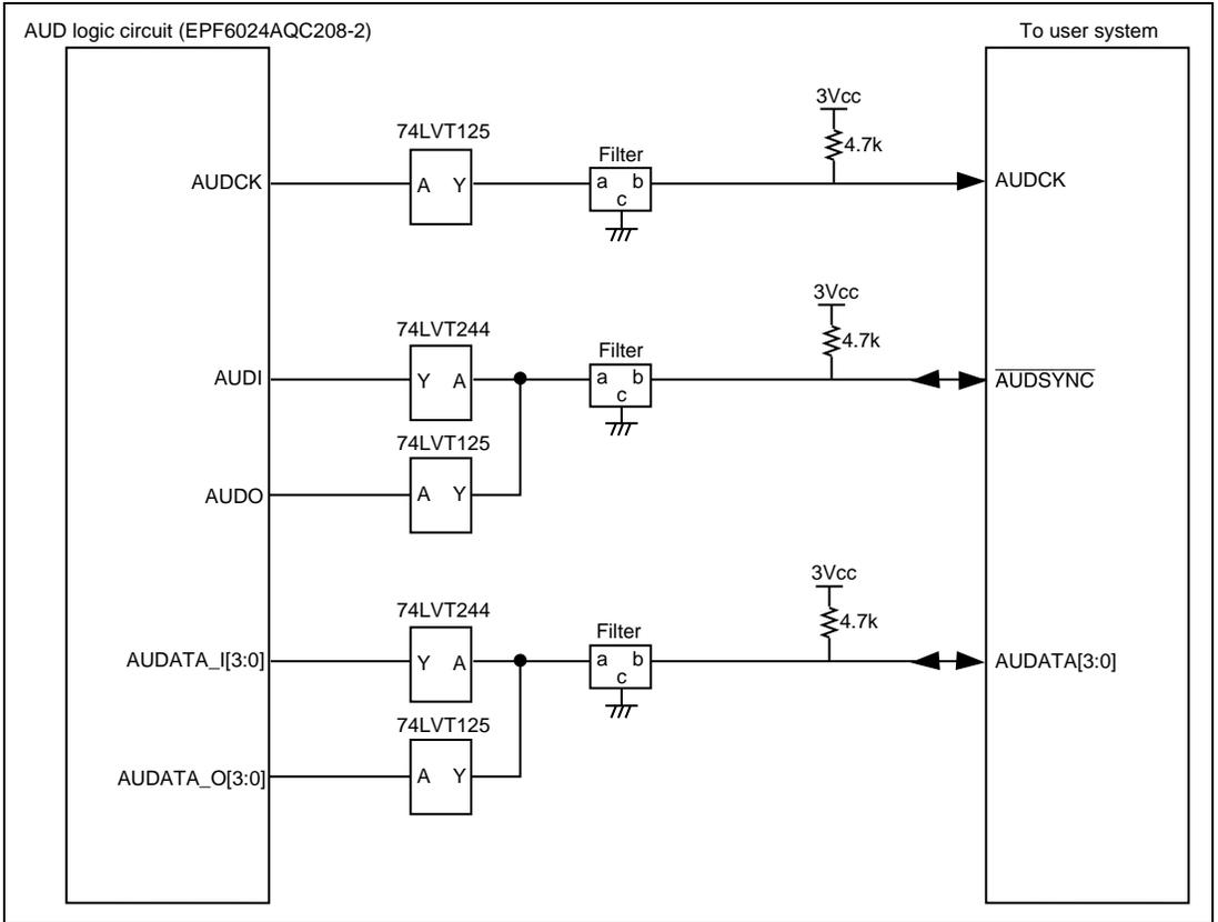
**Figure 6.9 User System Interface Circuit of the AUD Pin (HS7727KCI02H)
