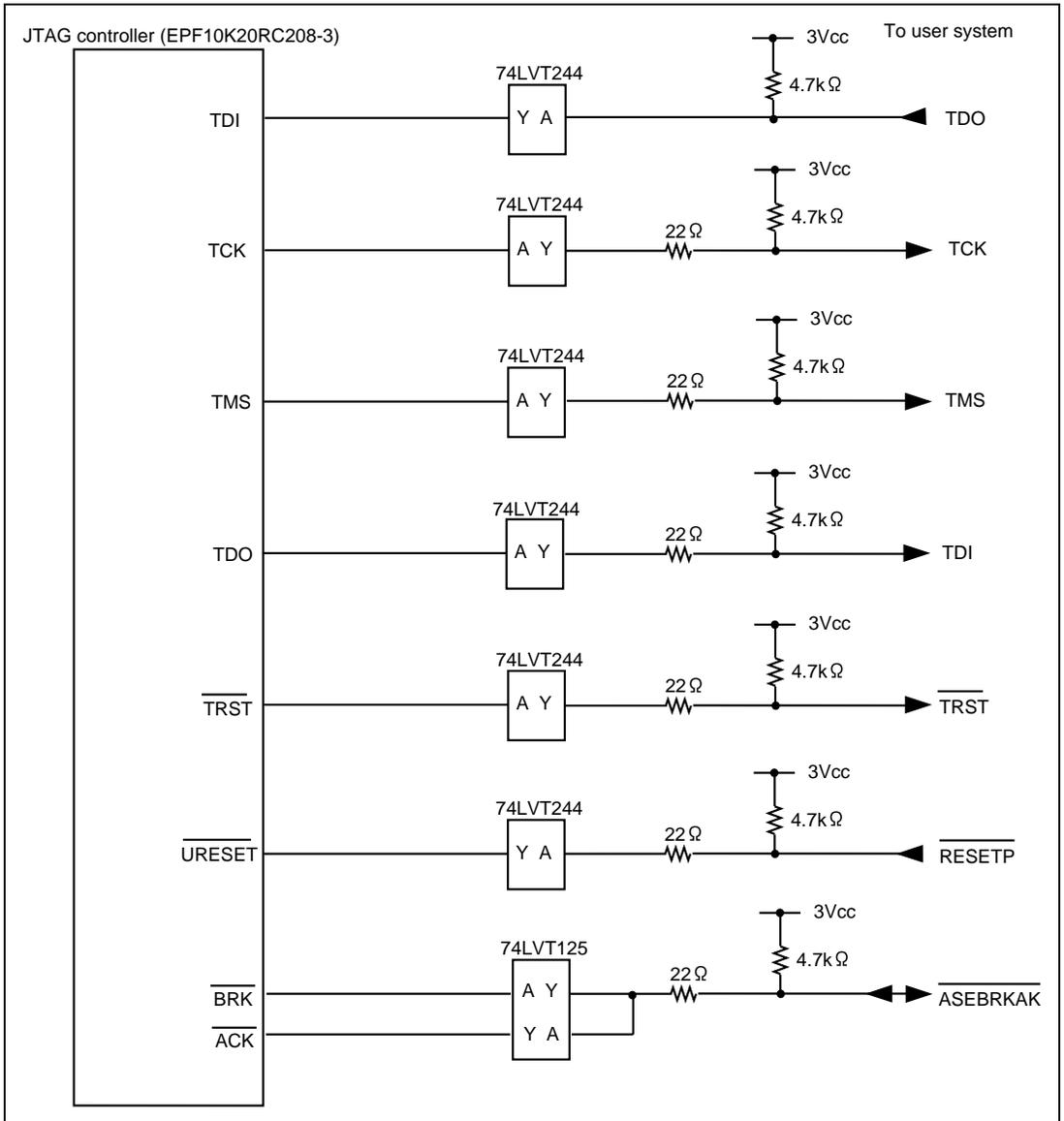
**Figure 6.7 User System Interface Circuit (HS7727KCI01H)
