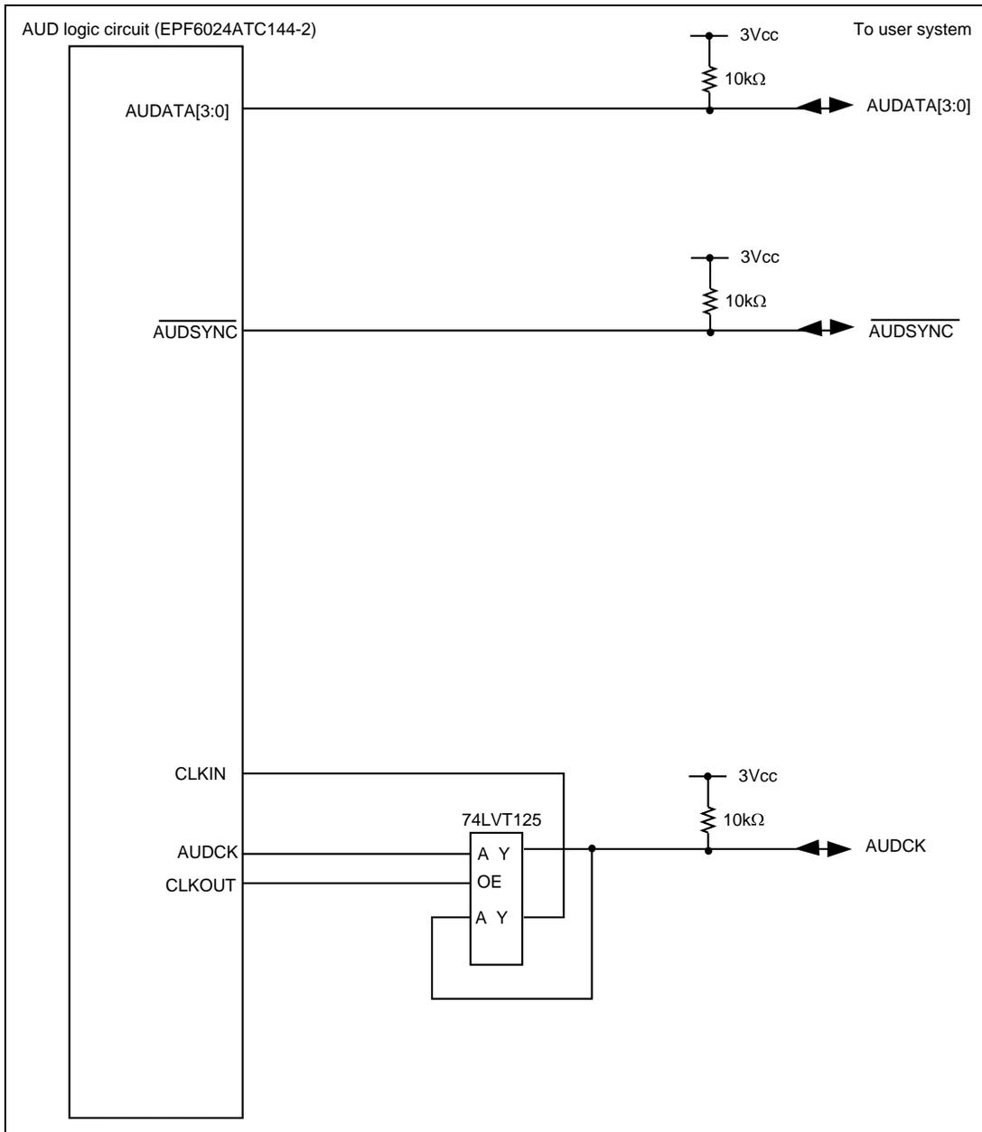
**Figure 6.6 User System Interface Circuit of the AUD Pin (HS7727KCM02H)
