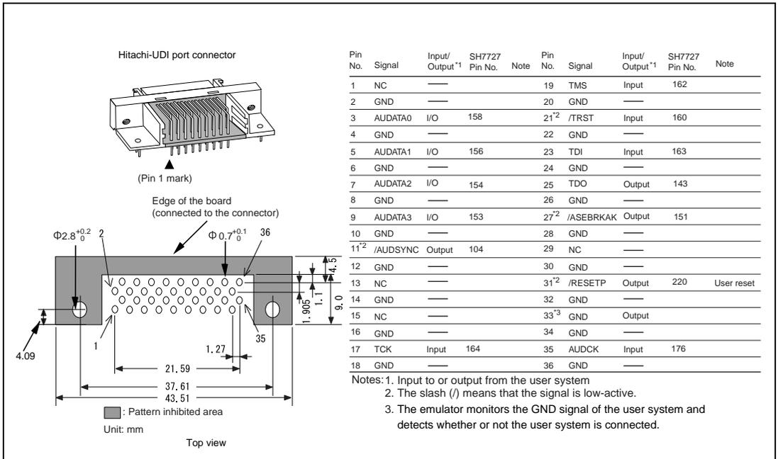
Figure 6.3 Pin Arrangement of the Hitachi-UDI Port Connector (36 Pins)
