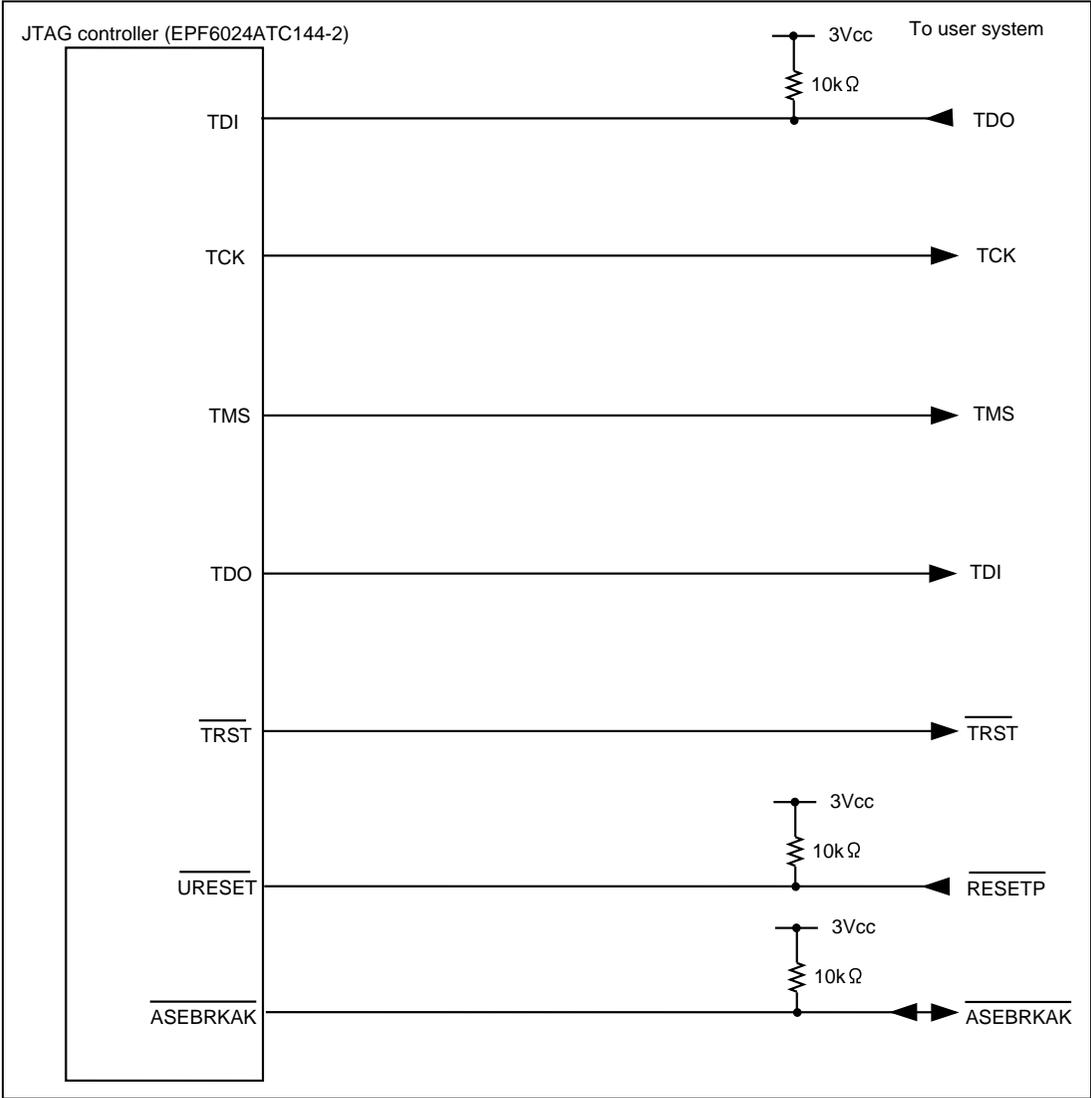
**Figure 6.5 User System Interface Circuit of the Hitachi-UDI Pin (HS7727KCM02H)
