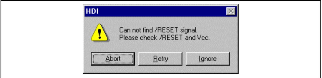
Figure 2.14 [Can not find /RESET signal] Dialog Box
