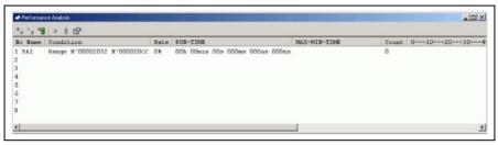
Figure 4.58 [Performance Analysis] Dialog Box (Setting Completed)
