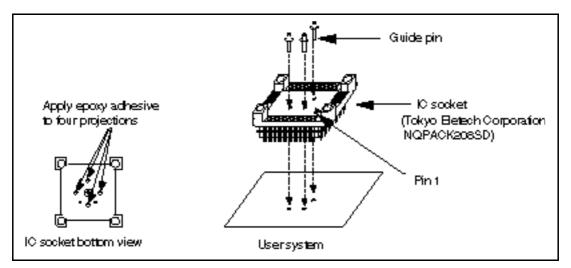
Figure 3 Installing IC Socket to User System
