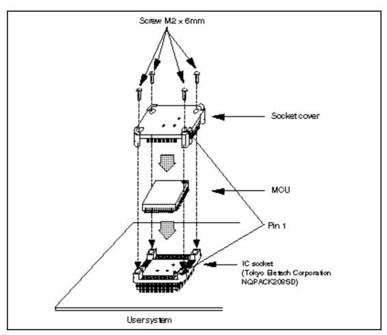
Figure 8 Installing MCU to User System
