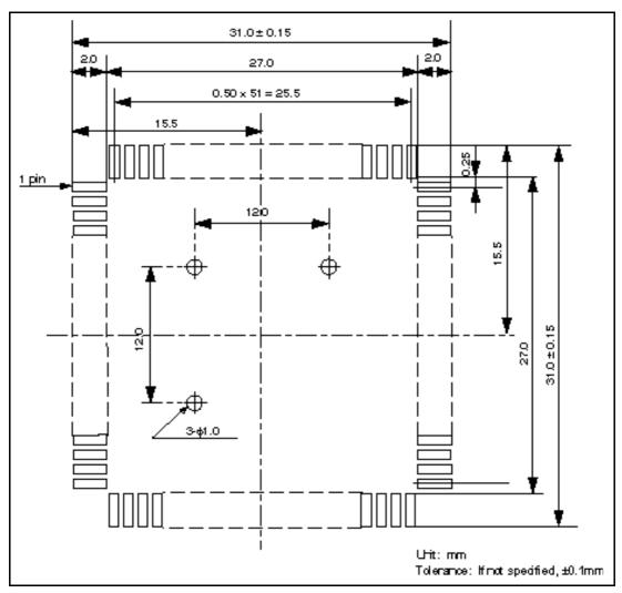
Figure 5 Recommended Dimensions for Mount Pad
