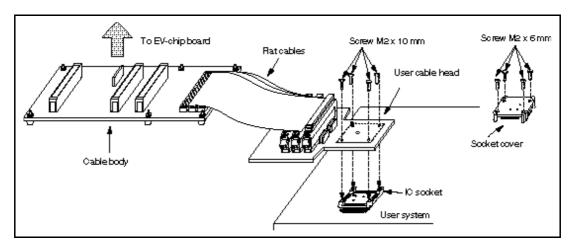
Figure 1 HS 7054ECH8 1H User System Interface Cable
