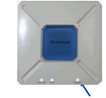
After the power is on, the TARGET LED lights up.
