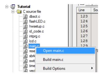
Place an event at the call to main(); by double clicking in the On-Chip Breakpoint column next to the line to stop at.
