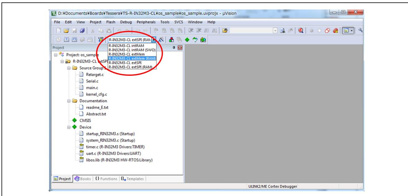
By pressing “Options for Target...” button, target settings can be customized/changed. For example, flash loader can be changed.
