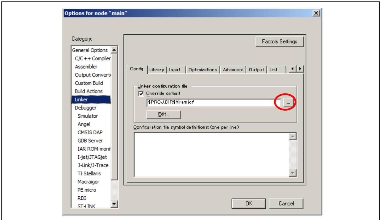
The R-IN32M3 board supports different boot options which can be selected via bit 1 and bit 2 of the MODE\_SW switch. To select one of this option you have to select the right linker parameter in the IAR environment. In the Linker Category on the left side of the [Project] / [Options...] menu use the [Config] tab in the right window and modify \*.icf file as shown below:
