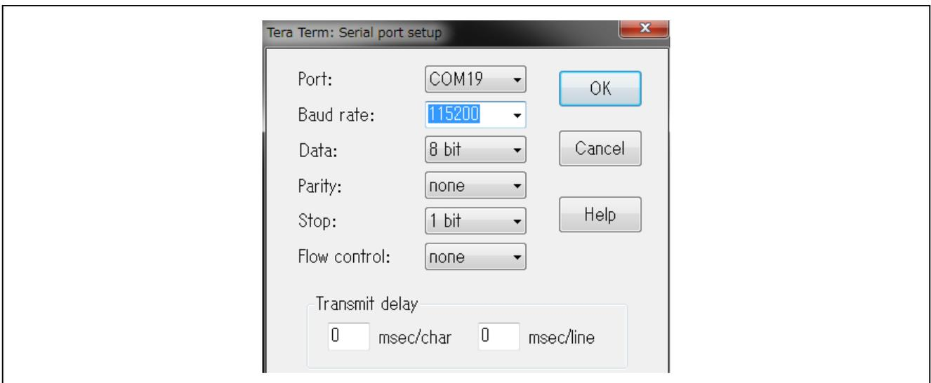
Set the baud rate to 115200, data to 8-bit, no parity, 1 stop bit, and no flow control.
