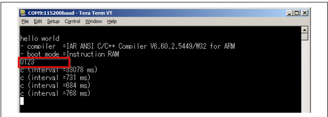
when you input “0”,”1”,”2”,”3” from serial terminal, Outputs level which are assigned at pins from 0 to 3 of CN20 of R-IN32M3 CL board are inverted.
