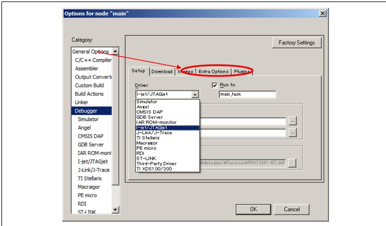
As an alternative to the I-jet debugger you can use other debuggers as well, which are supported by the IAR Embedded Workbench. To modify the debugger type you have to switch to the [Project] → [Options ...] dialog and select the category [Debugger]. Please click in the drop down menu the debugger you want to use and click [OK].
