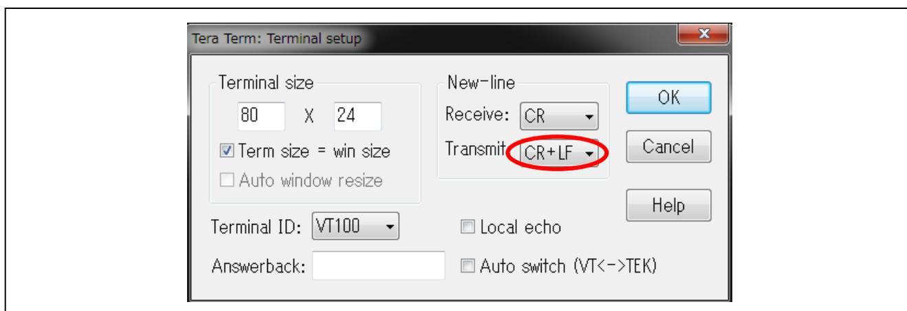
Please set the terminal software to transmit “CR+LF” for new lines (In TeraTerm the option is [Transmit] under [New-line] in [Terminal setup] as shown above.)
