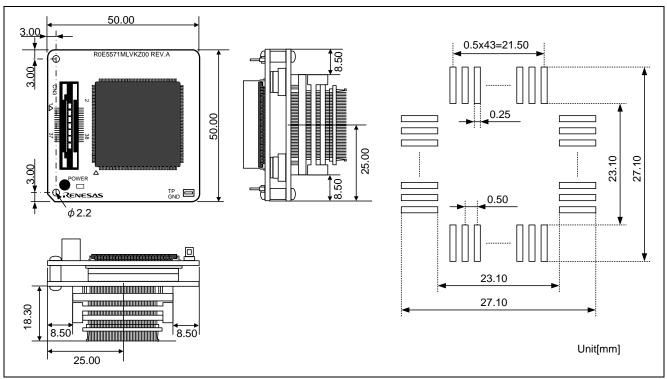
Figure 4 Reference Foot Pattern and Dimensions of This Product (R0E5571MLDMB00)
