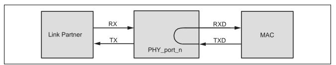
Figure 2.4 Near-End Loopback Diagram
