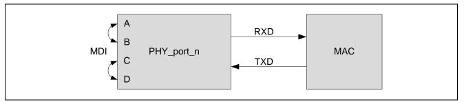
Figure 2.5 Connector Loopback Diagram
