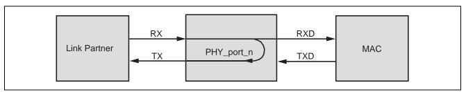
Figure 2.3 Far-End Loopback Diagram
