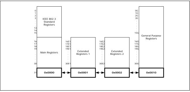
Figure 3.1 Register Space Diagram
