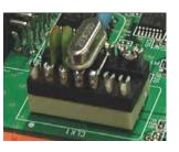
Figure 2-3. Oscillator Shape
