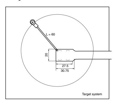
Figure 2-9. Where GND Wire Can Be Connected
