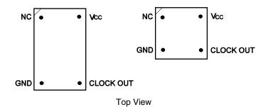
Figure 2-4. Mapping of Oscillator to Socket
