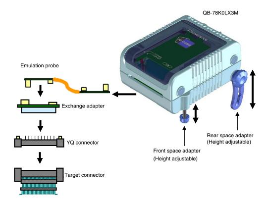
Figure 2-10. Connection Using Emulation Probe
