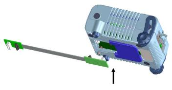
Insert CN1 and CN2 of the probe into TCN1 and TCN2 of the QB-78K0LX3M.
