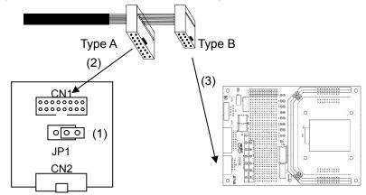
Figure 2-8. Connection Diagram When Using IIC/78K0S/KX1+ Adapter
