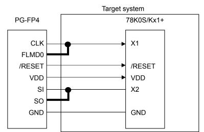
Figure 2-10. Connection Diagram
