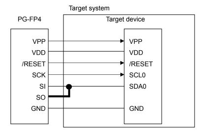
When I<sup>2</sup>C communication mode is used and the IIC/78K0S/KX1+ adapter is used, shorting the SI pin and SO pin in the target system is not required.
