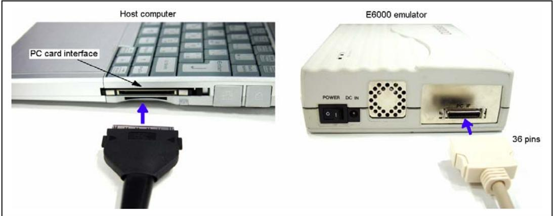
**Figure 2 Connecting the PC Card Interface to the E6000 Emulator**
