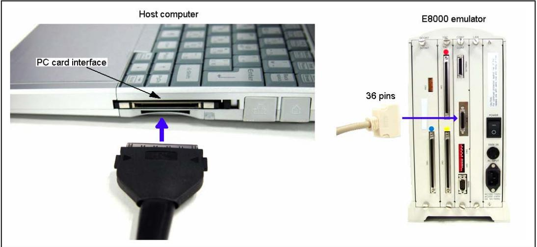
**Figure 4 Connecting the PC Card Interface to the E8000 Emulator**
