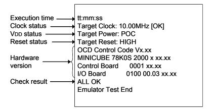
• Execution time: The time when checking was started by clicking the [Test] button.
