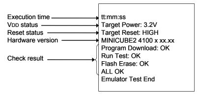
• Execution time: The time when checking was started by clicking the [Test] button
