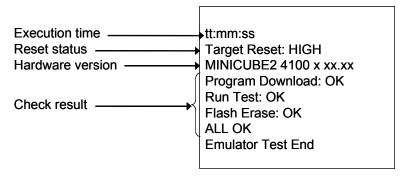
• Execution time: The time when checking was started by clicking the [Test] button
