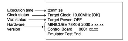
In this NG example, the error "Target Power: OFF" is detected.
