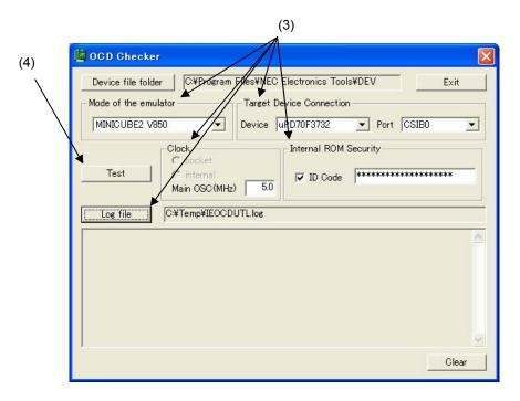
(5) When all of the tests are complete, the result dialog box is displayed as shown below. The contents displayed in the log view window are saved in the log file. If an NG is displayed, refer to 4.3 Error Output and 4.4 Action for Error.
