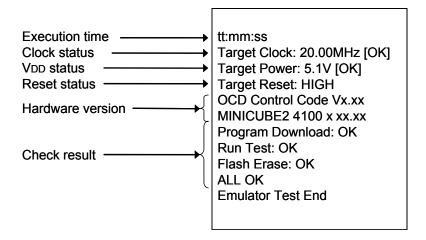
• Execution time: The time when checking was started by clicking the [Test] button
