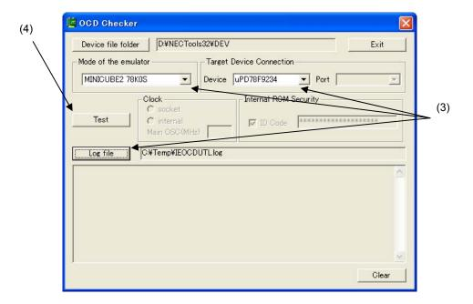
(5) When all of the tests are complete, the result dialog box is displayed as shown below. The contents displayed in the log view window are saved in the log file. If an NG is displayed, refer to 5.3 Error Output and 5.4 Action for Error.
