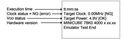
In this NG example, the clock status 0.00MHz is detected as an error.
