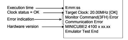
In this NG example, the monitor command (3FH) error and communication error are output.
