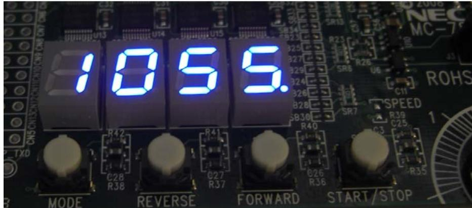
To start the motor, press the START/STOP pushbutton. To stop the motor, press START/STOP again. During the motor operation, you can set the RPM to the desired speed using the SPEED potentiometer. Pressing MODE/DIRECTION during operation will toggle the display between the reference RPM and the actual measured RPM. Changing the direction can be done while the motor is running. The motor will ramp down and stop for a brief time and will ramp up in the opposite direction to the same set RPM.
