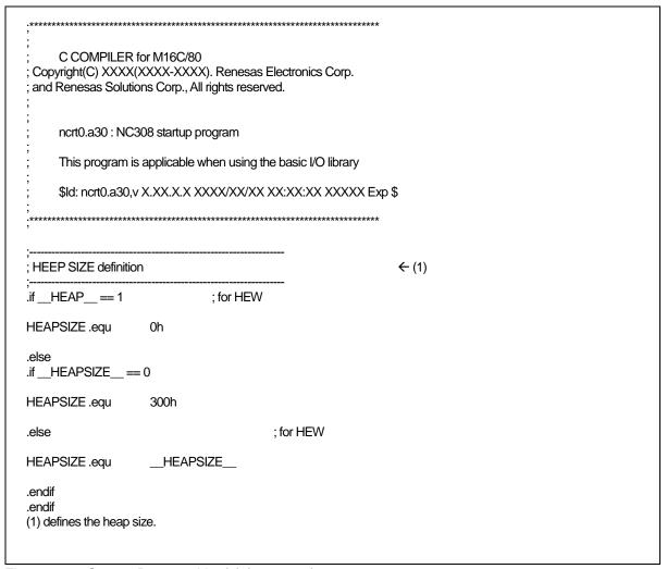
Figure 2.6 Startup Program List (1) (ncrt0.a30)
