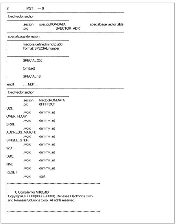
Figure 2.26 Listing of sect308.inc in Single-Chip Mode (4)
