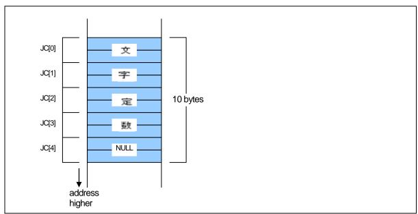
Figure B.46 Memory Location of wchar\_t Type Character Constant Assigned Array
