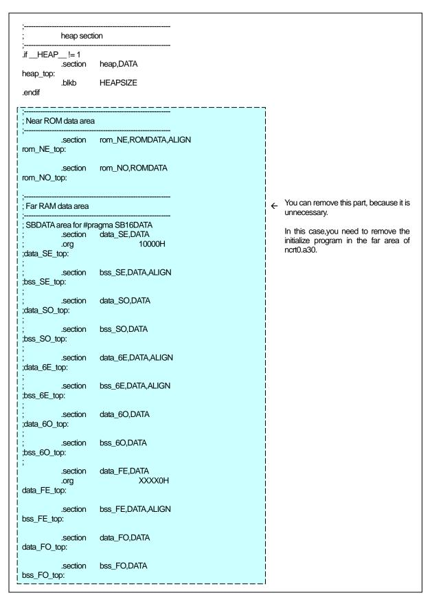
Figure 2.24 Listing of sect308.inc in Single-Chip Mode (2)
