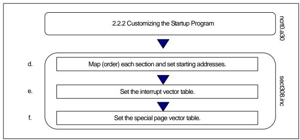
Figure 2.21 Example Sequence for Modifying Startup Programs
