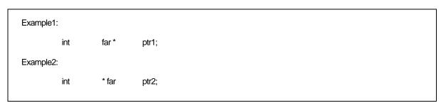
Figure B.7 Example of Declaring a Pointer Type Variable (1)
