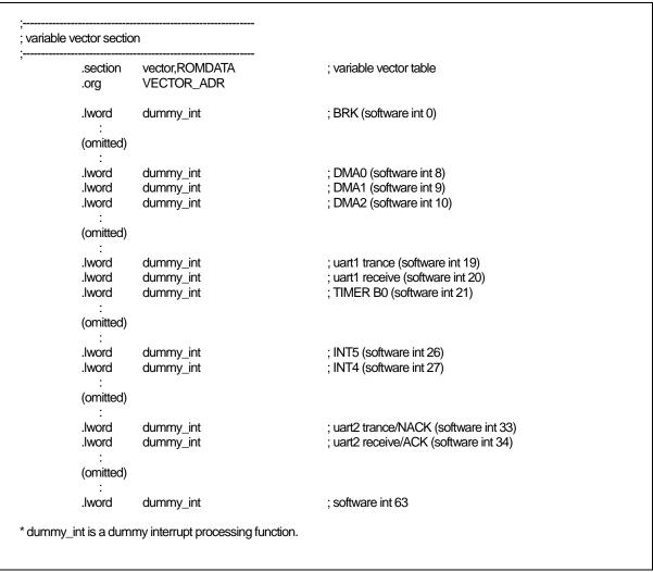
Figure 2.27 Interrupt Vector Address Table
