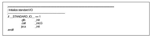
Figure 2.13 Part of ncrt0.a30 Where init Function is Called
