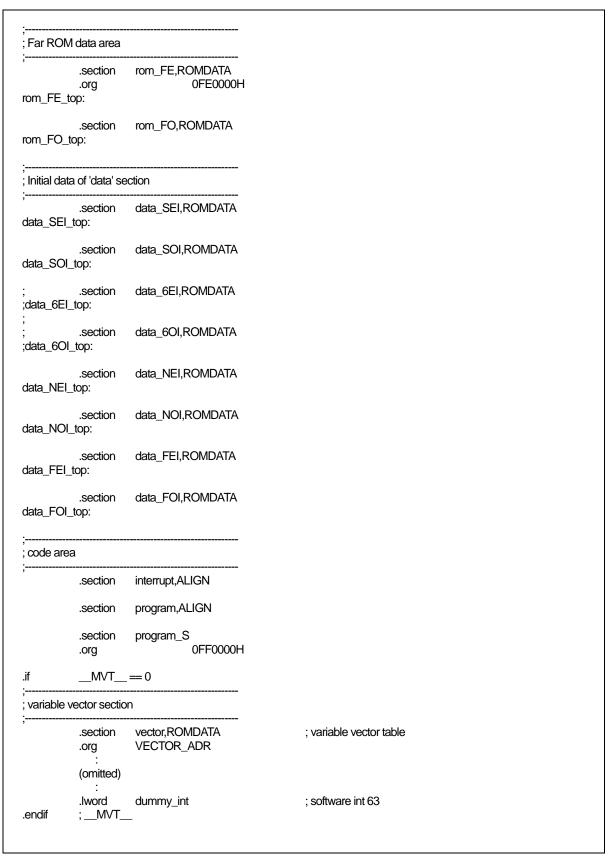
Figure 2.25 Listing of sect308.inc in Single-Chip Mode (3)
