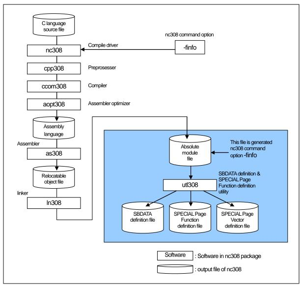
Figure G.1 NC308 Processing Flow
