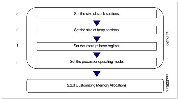
Figure 2.12 Example Sequence for Modifying Startup Programs
