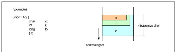
Figure D.6 Example of Placement of Union
