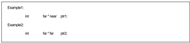
Figure B.8 Example of Declaring a Pointer Type Variable (2)
