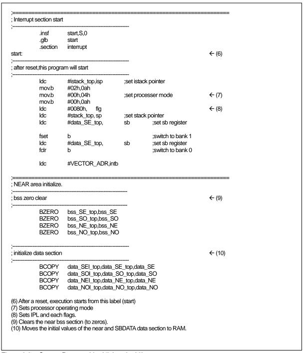
Figure 2.9 Startup Program List (4) (ncrt0.a30)
