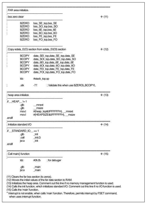
Figure 2.10 Startup Program List (5) (ncrt0.a30)
