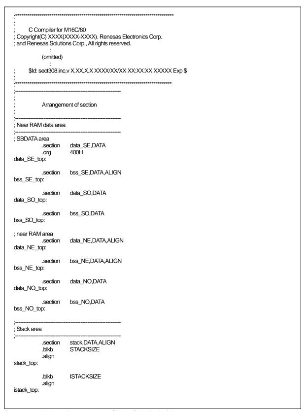
Figure 2.23 Listing of sect308.inc in Single-Chip Mode (1)
