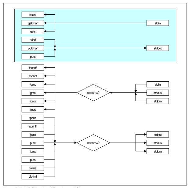
Figure E.3 fRelationship of Functions and Streams
