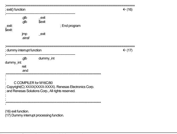
Figure 2.11 Startup Program List (6) (ncrt0.a30)
