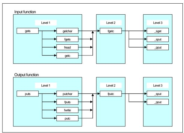
Figure E.1 Calling Relationship of I/O Functions
