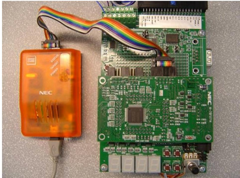
Figure 8-3 OCD Debugger Unit Connection
