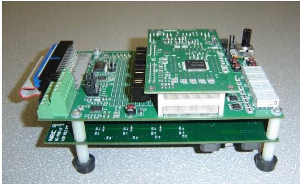
**Figure 3-1 MC-LV-KIT-714 Kit Configuration**
