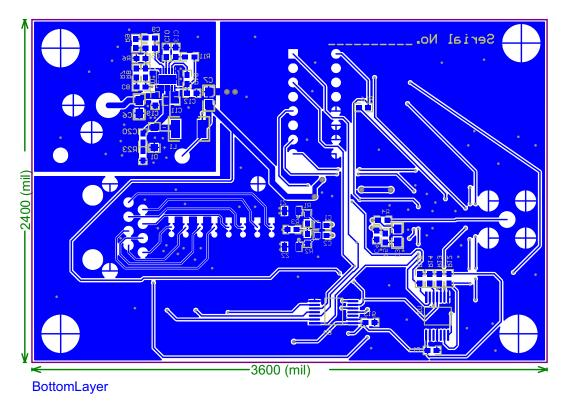
FIGURE 4. PCB BOTTOM LAYER WITH SILKSCREEN
