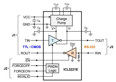
Figure 2. Functional Block Diagram of ICL3221E
