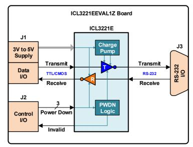
Figure 1. ICL3221EEVAL1Z Board Block Diagram
