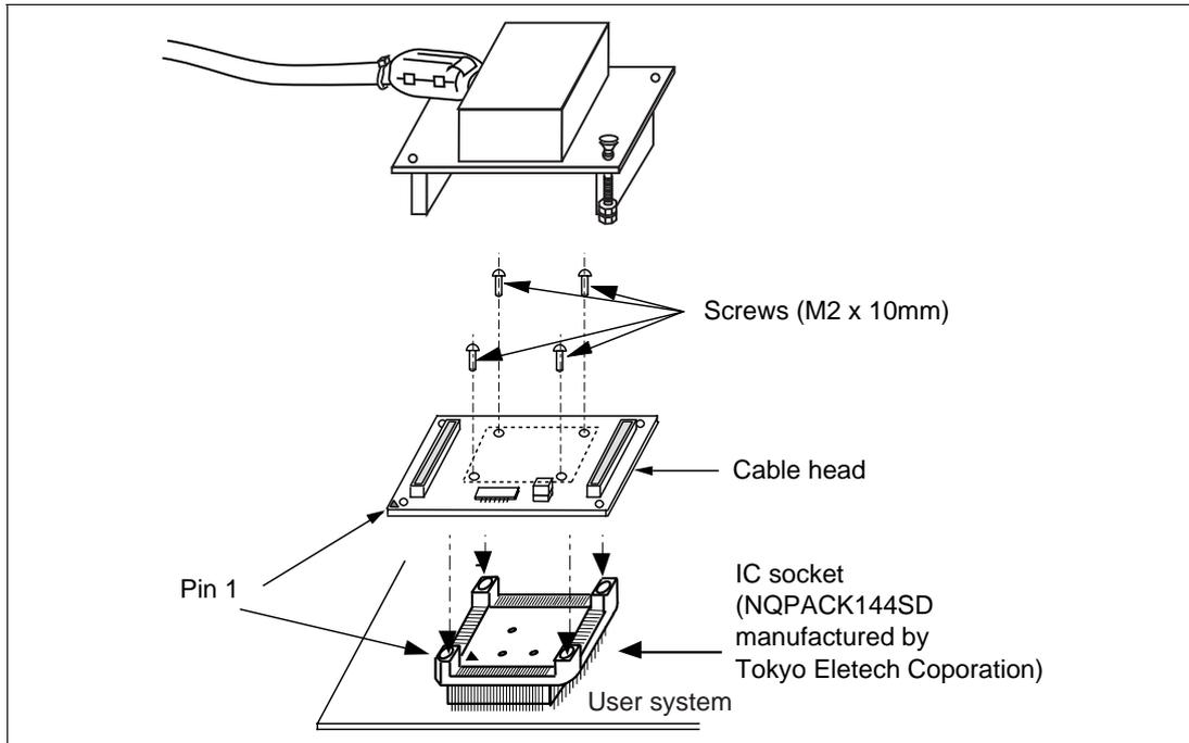
**Figure 4 Connecting User System Interface Cable to User System**
