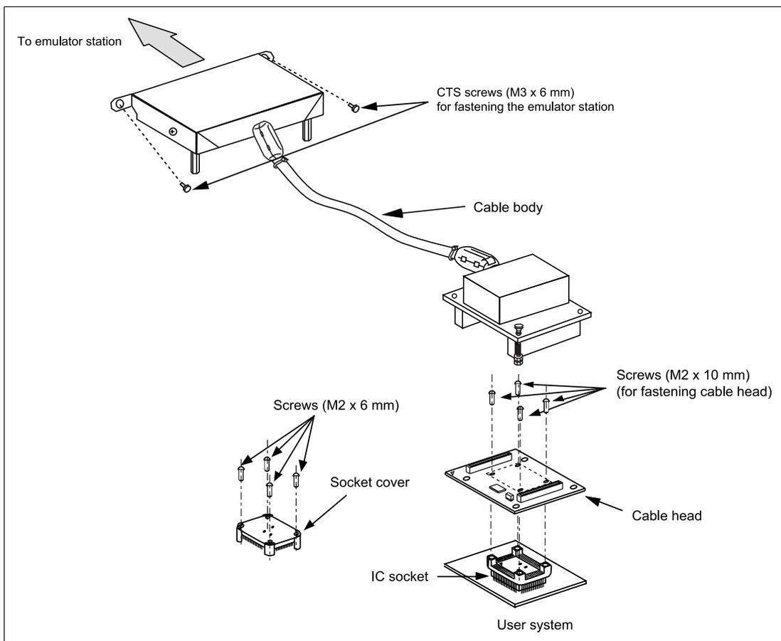
Figure 1 HS2556ECH61H User System Interface Cable
