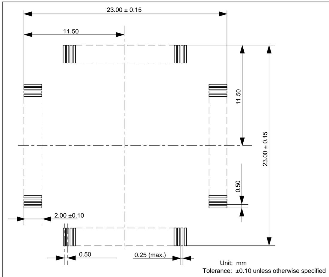
Figure 6 Recommended Dimensions for Mount Pad
