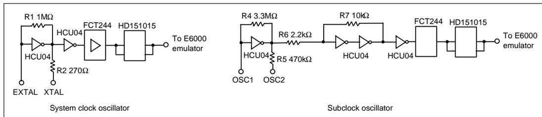
**Figure 10 Clock Oscillator Circuits**
