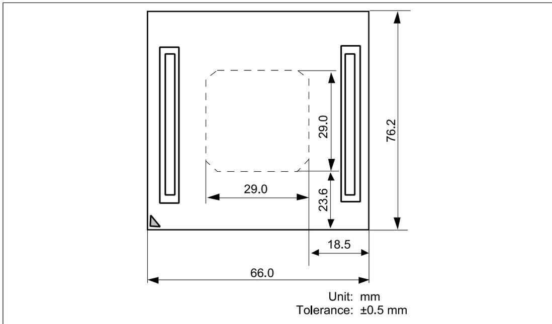
Figure 7 Dimensions for User System Interface Cable Head
