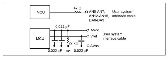
Figure 2.4 User System Interface Circuit for AN0 to AN7, AN12 to AN15, DA0 to DA3, AVcc, AVss, and Vref Signals
