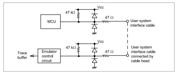
Figure 2.5 IRQ0-IRQ7 and WAIT User System Interface Circuit
