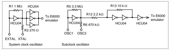
Figure 10 Clock Oscillator Circuits
