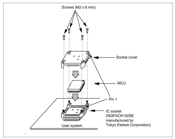
Figure 9 Installing MCU to User System
