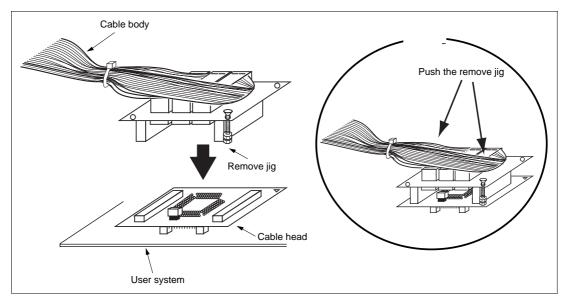
Figure 5 Fastening Cable Body
