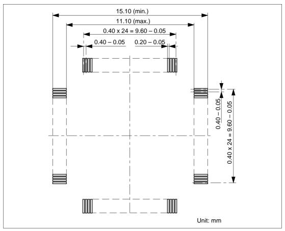
Figure 6 Recommended Dimensions for Mount Pad
