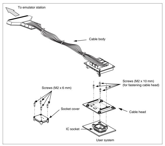
Figure 1 HS2237ECN61H User System Interface Cable
