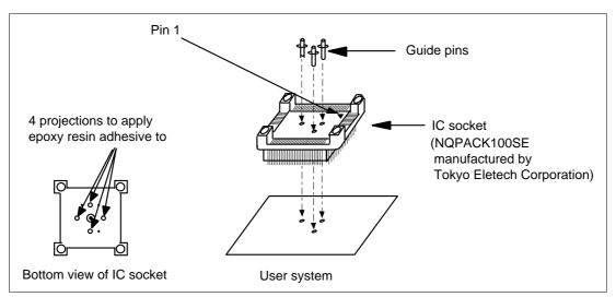
Figure 3 Location Setting of IC Socket
