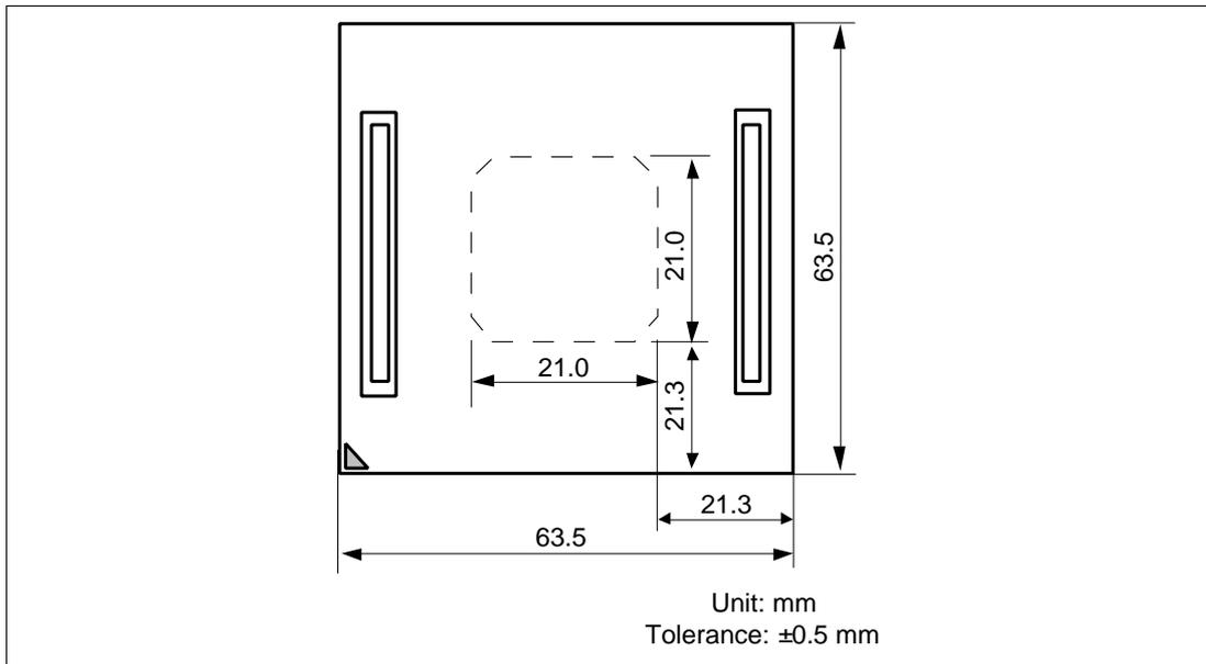
**Figure 8** Dimensions for User System Interface Cable Head
