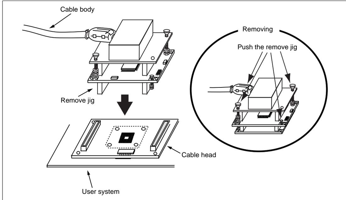
**Figure 6 Fastening Cable Body**
