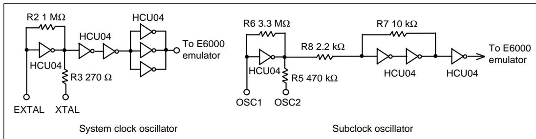
**Figure 12 Clock Oscillator Circuits**
