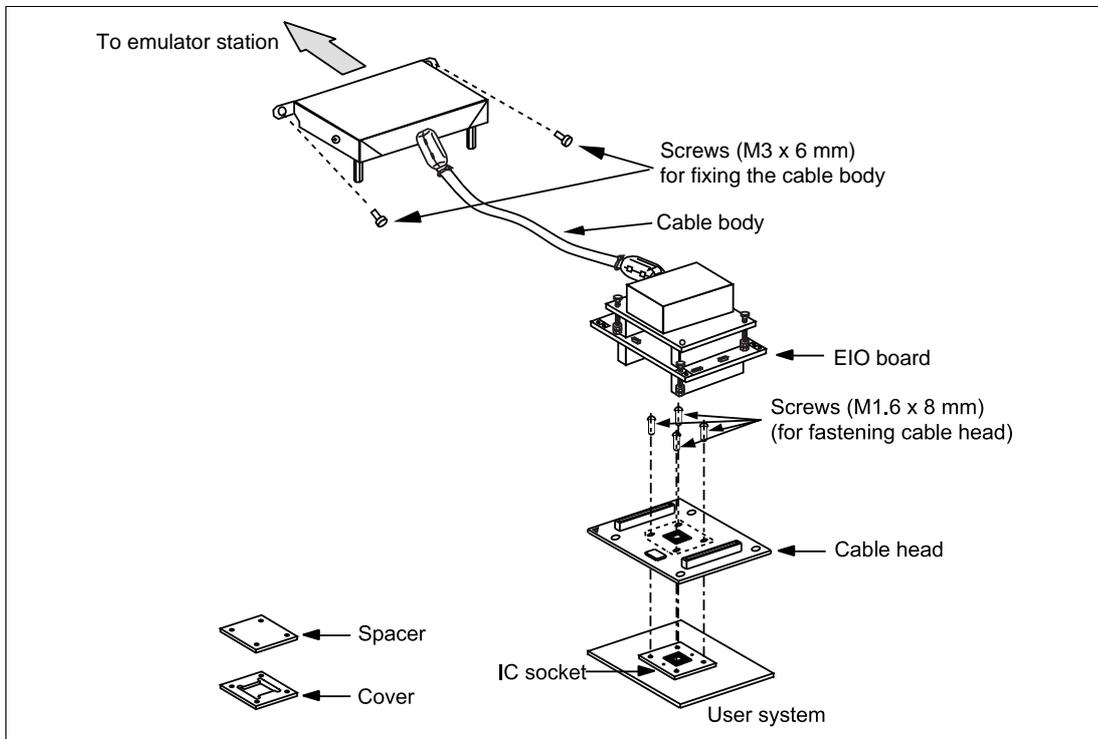
**Figure 1 HS2218ECB62H User System Interface Cable**
