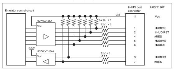
Figure 6.7 Interface Circuit in the Emulator (Reference)
