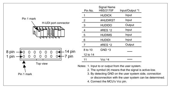
Figure 6.1 Pin Arrangement of the H-UDI Port Connector (14-Pin Type)
