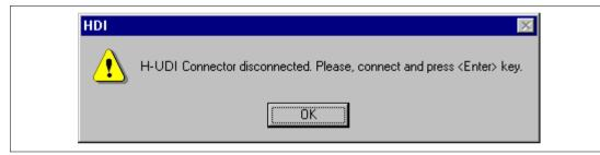
Figure 2.11 [H-UDI Connector Disconnected] Dialog Box
