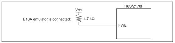
Figure 6.6 Connection of the FWE Pin
