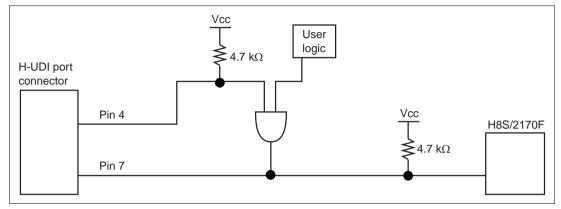
Figure 6.5 Connection of the #RES Pin
