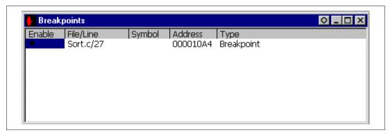
Figure 3.37 [Breakpoints] Window (Software Breakpoint Setting)
