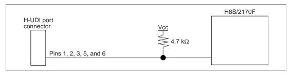
Figure 6.3 Connection of Emulator and the MCU
