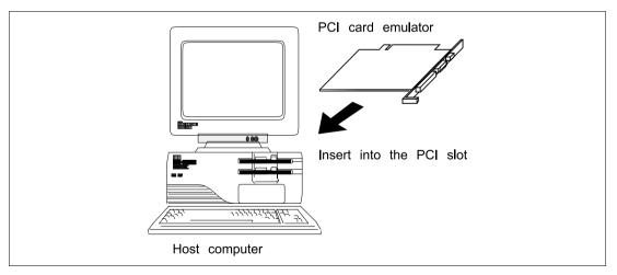
Figure 2.3 Inserting the PCI Card Emulator into the Host Computer
