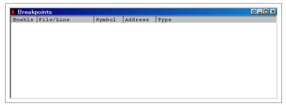
Figure 3.33 [Breakpoints] Window (Before Software Breakpoint Setting)
