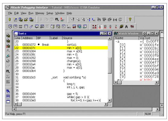
Figure 3.27 [Program] Window (Step Out)
