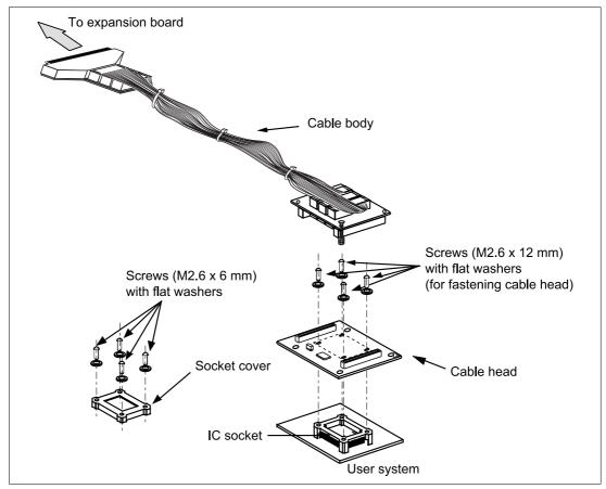
Figure 1 HS3937ECH61H User System Interface Cable
