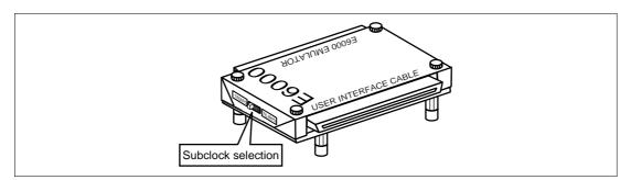
Figure 9 Expansion I/O board Subclock Selection
