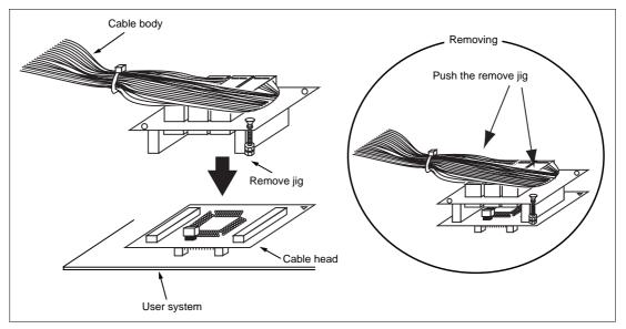
Figure 4 Fastening Cable Body
