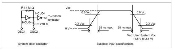
Figure 11 System Clock Oscillator and Subclock Input Specifications
