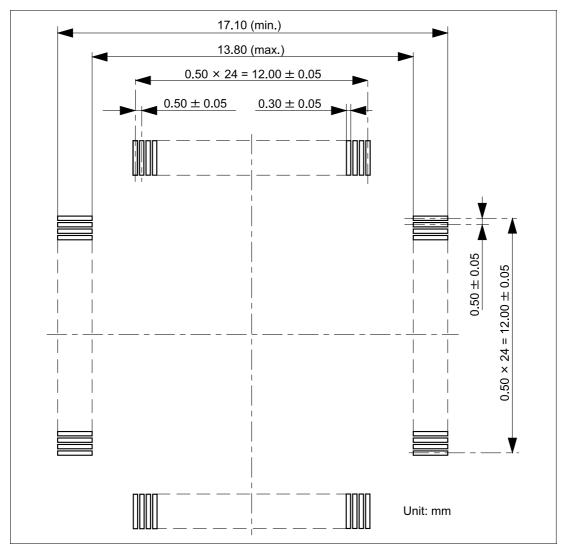
Figure 5 Recommended Dimensions for Mount Pad
