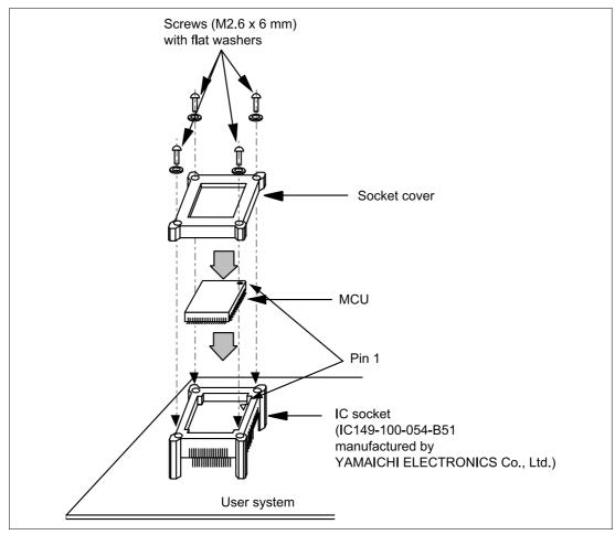
Figure 8 Installing MCU to User System
