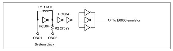
Figure 9 Oscillator Circuit
