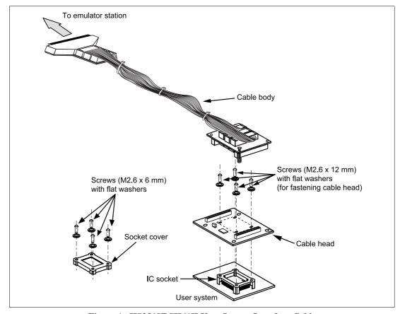
Figure 1 HS2318ECH61H User System Interface Cable
