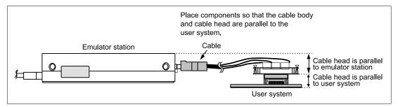
Figure 10 User System Interface Cable Location Example
