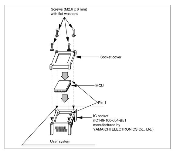
Figure 8 Installing MCU to User System
