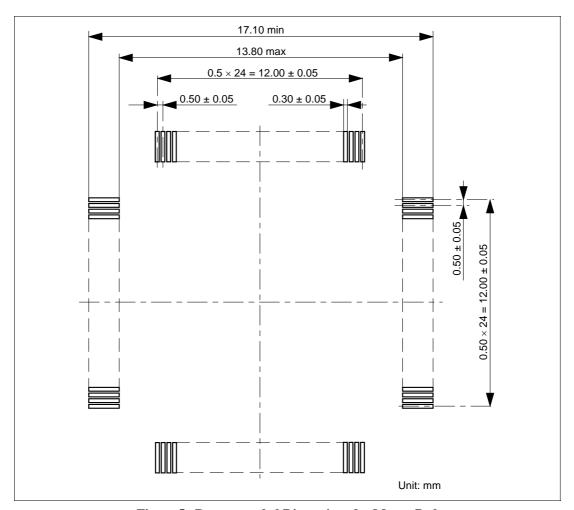
Figure 5 Recommended Dimensions for Mount Pad
