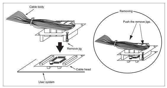
Figure 4 Fastening Cable Body
