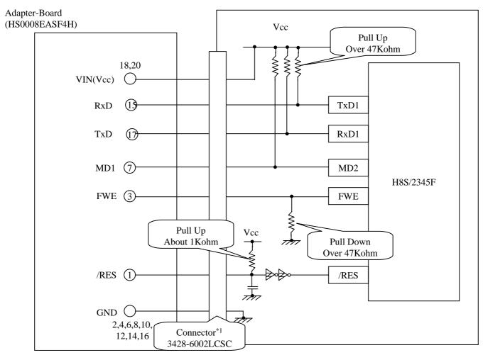
Setting the switches on the HS0008EASF4H on using H8S/2345F
