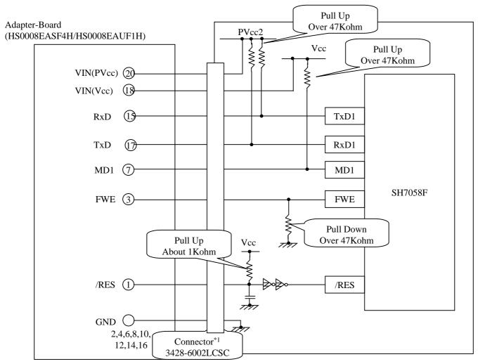
Setting the switches on the HS0008EASF4H on using SH7058F
