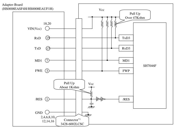
Setting the switches on the HS0008EASF4H on using SH7046F
