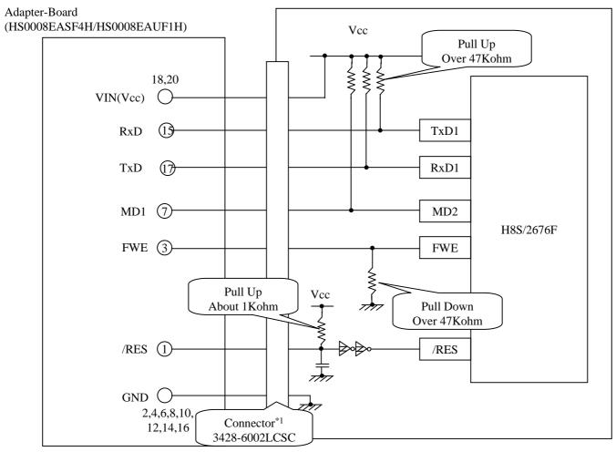
Setting the switches on the HS0008EASF4H on using H8S/2676F
