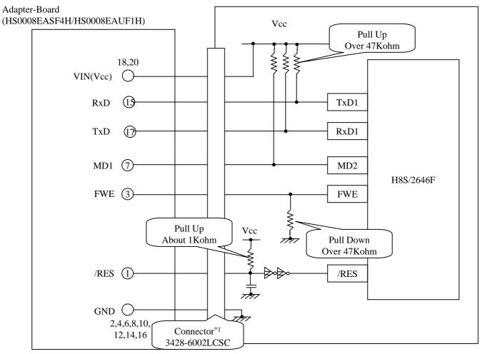
Setting the switches on the HS0008EASF4H on using H8S/2646F
